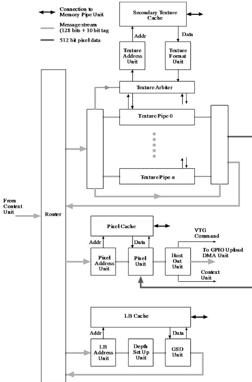
Figure 1.3 Rasterizer Block Diagram
