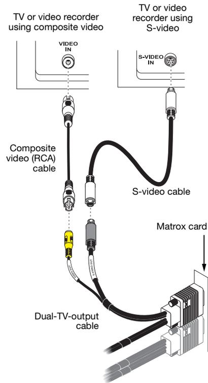
(Note: Using the Matrox composite video **and** S-video connectors at the same time is optional.)
