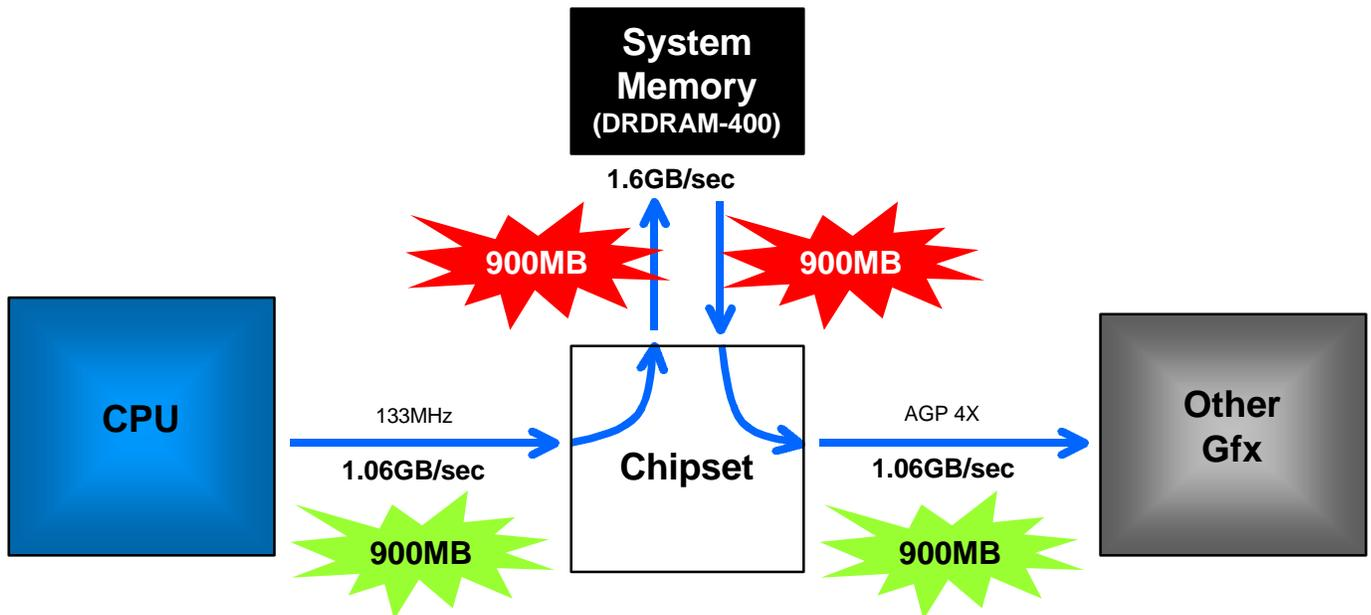
In this case, the graphics controller does not implement Fast Writes. This causes the CPU to stall while it waits for the data to be transferred over the system. Even with 1.6 GB/sec, the system memory bus is unable to handle the constant shuffling of 900MB/sec data in and out of system memory. This thrashing on the system memory bus will also cause overall system performance to degrade.
