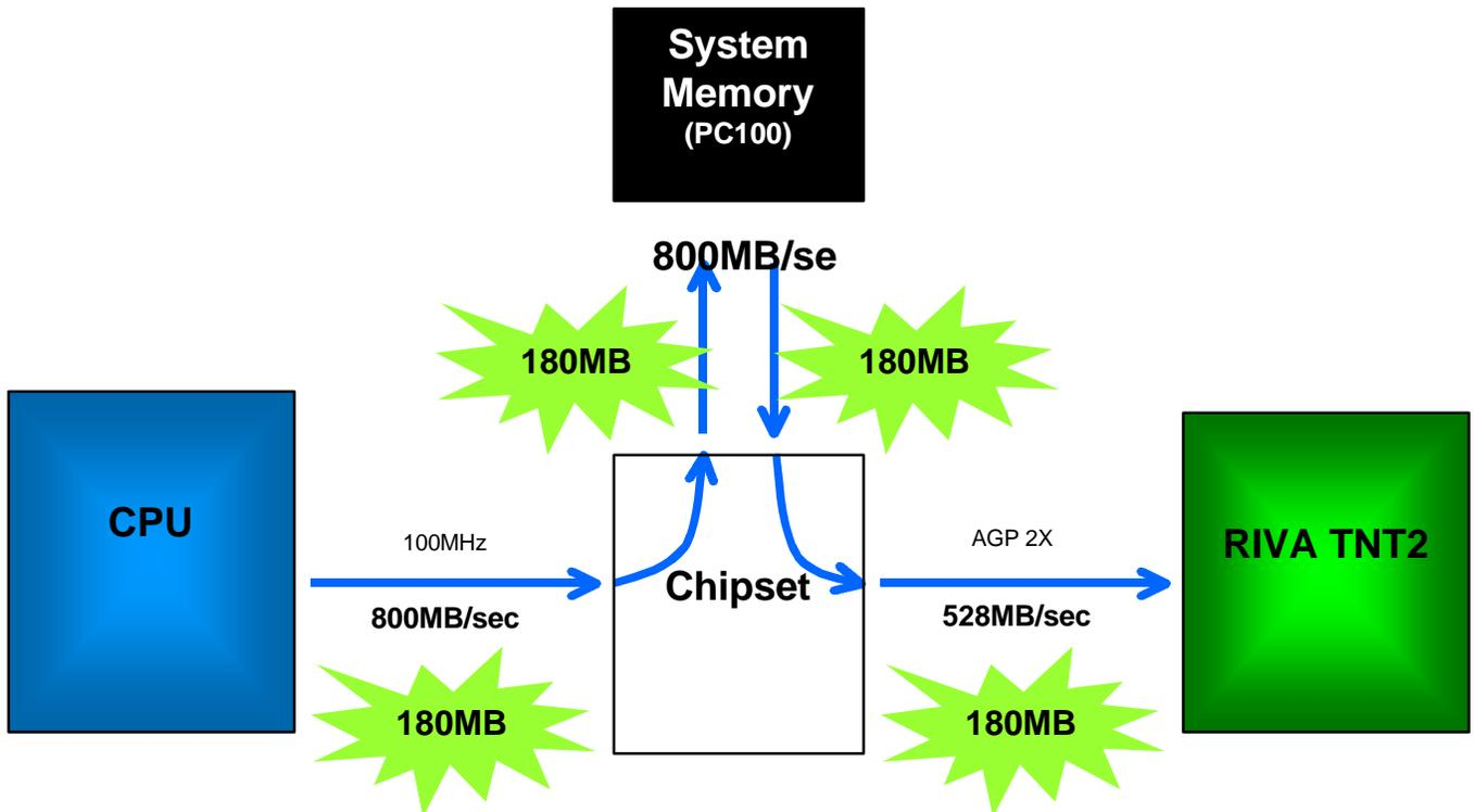
However, next-generation 3D applications will need up to five times greater triangle performance. This means that for the same triangle size (in terms of bytes transferred per triangle, e.g. 90 Bytes/triangle), the required bandwidth for data transfers will increase five times or up to 900 MB/sec! This exceeds the bandwidth of the current system.
