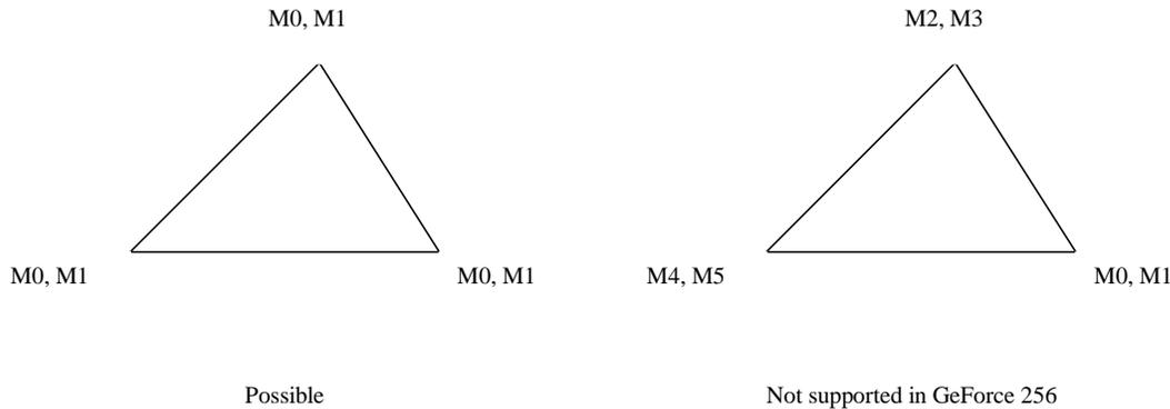
The GeForce 256 supports 2 blending matrices per vertex. These are not divisible within a triangle. In Direct3D, blending matrices are applied on a per vertex basis and cannot be changed on a per primitive basis – in other words, you cannot reassign the blending matrices within a Draw\*Primitive\* call. If you require more sophisticated vertex blending than this, you have several options
