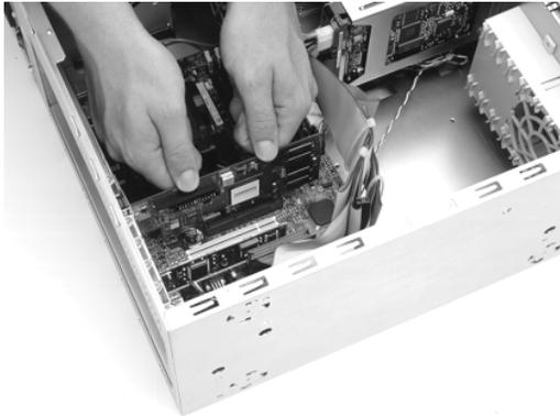
6. Once you are certain that the card is installed properly in its slot, secure it to the computer frame with the screw you removed in step 2. Make sure the card does not lift out of the AGP slot while tightening the bracket screw.
