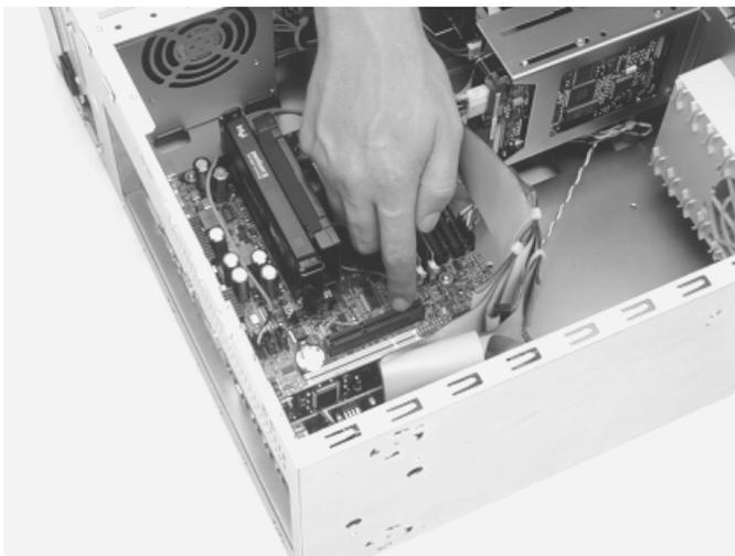
2. Remove the screw attached to the bracket cover and remove the bracket plate.
