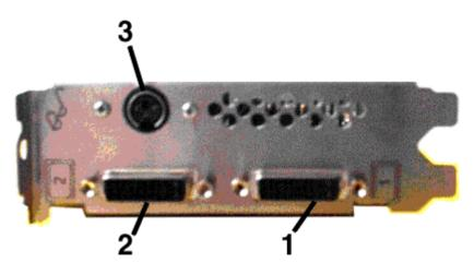
**Note:** If the connector on your stereoviewing eyewear does not fit into the Mini-DIN connector on the card, please contact your supplier or the manufacturer of the stereo glasses for information on how to obtain an adapter cable.
