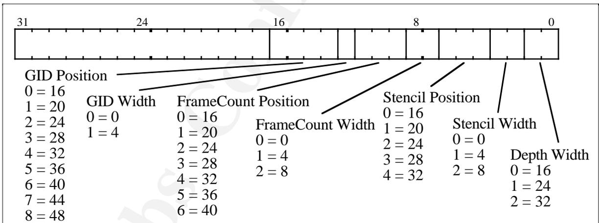
It is still possible to part populate the local buffer so other combinations of the field widths are possible (i.e. depth field width of 0), however this may give problems if texture maps are to be stored in the local buffer as well.
