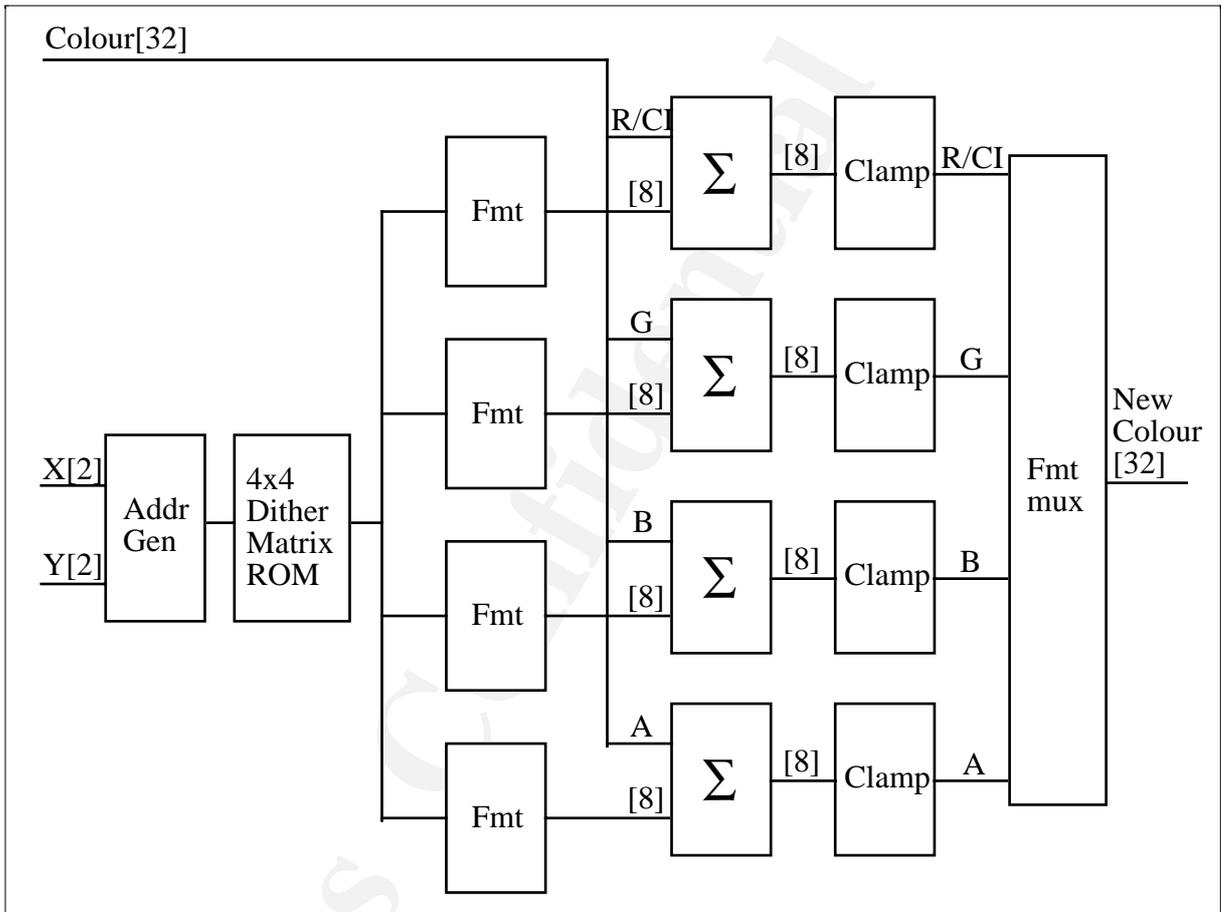
The dither matrix is held in a 4x4 array, indexed by the two bit values of X' and Y' (output from the Addr Gen block):
