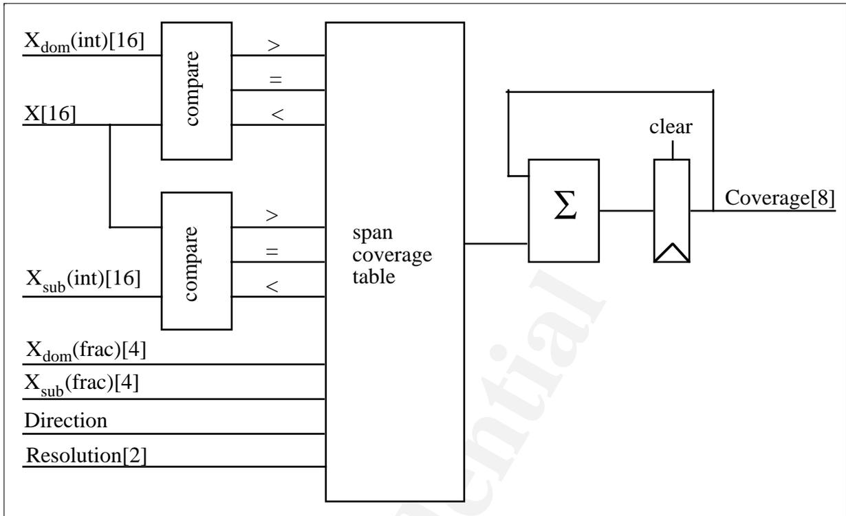
The coverage for to each sub scanline, at position  $X$ , is determined using the following table. Note the resolution (i.e. the number of sub pixel sample points in  $X$ ) is set to 4 in the table. We may want to allow a range of resolutions to give a quality vs. speed trade off, however this should be balanced with how fast we can blend pixels in the Alpha Blend Unit.
