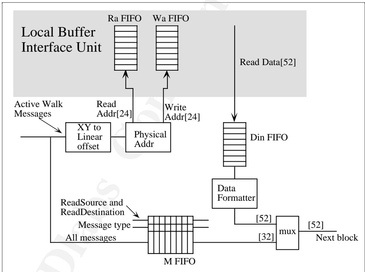
The actual reading of the memory and request arbitration is done in the Local Buffer Interface Unit.
