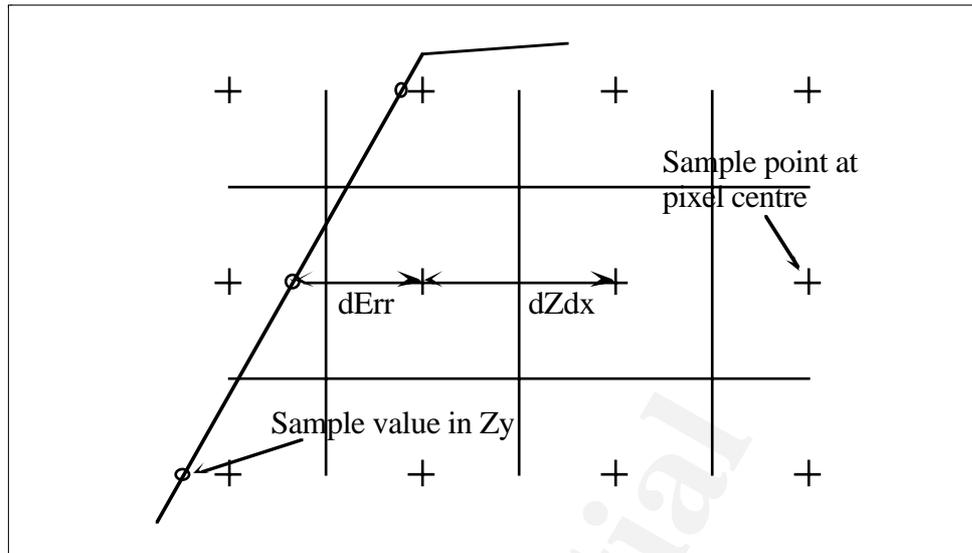
The start value has already been compensated to move it to the centre of a pixel in the Y directions. This only needs to be done once per triangle and is done in software. As the DDA is stepped in Y along the dominant edge the value of the interpolated parameter is calculated at the points marked by circles, whereas the value is required in the pixel's centre.
