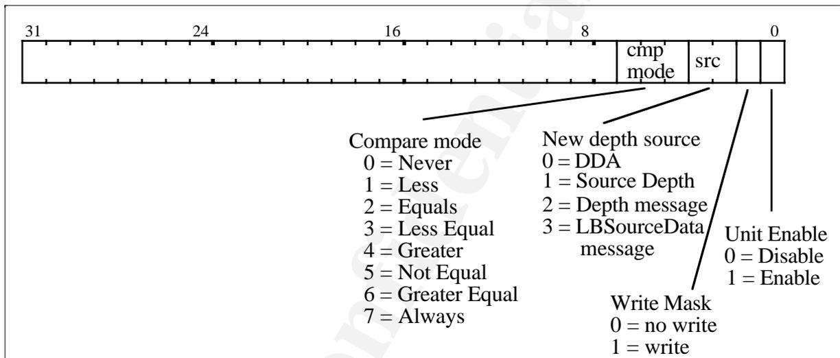
The single bit write mask enables or disables the updating of all the depth bits in the local buffer. The write masking is done by read-modify-write operations to the local buffer and not by controlling the write enables to the memories.
