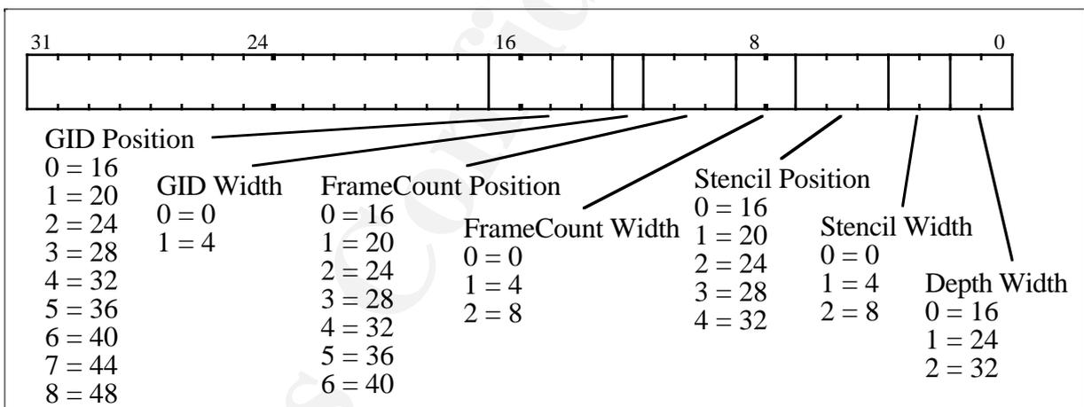
If the LBWriteFormat is erroneously set up such that two or more fields select the same bits in the local buffer then the highest priority field determines the value of the local buffer bits. The priority of the fields is (from highest to lowest) depth, stencil, frame count and then GID.
