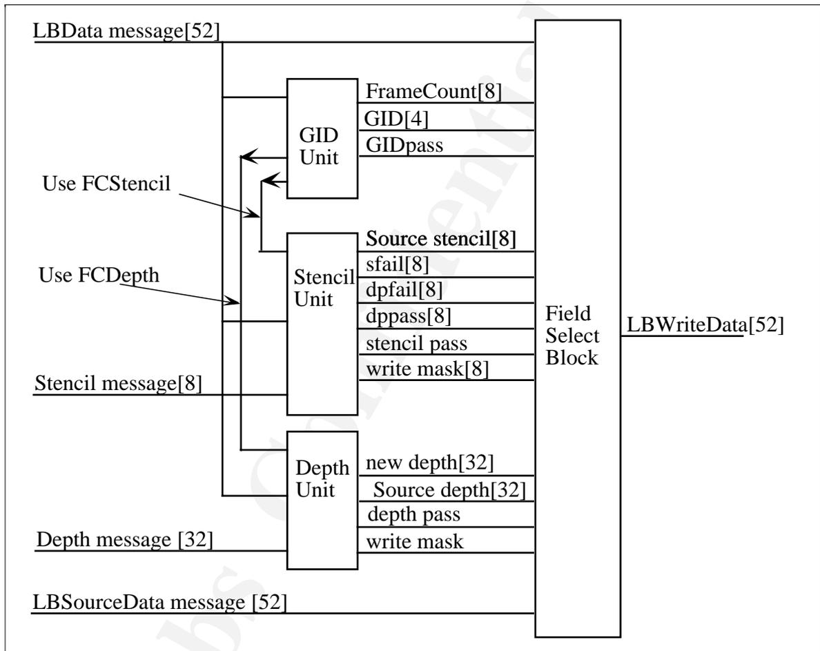
This diagram shows the three units working in parallel, however there are dependencies between the units. These dependencies are handled by the field select block and this selects either the original input values or the values generated by the individual blocks. This is described later.
