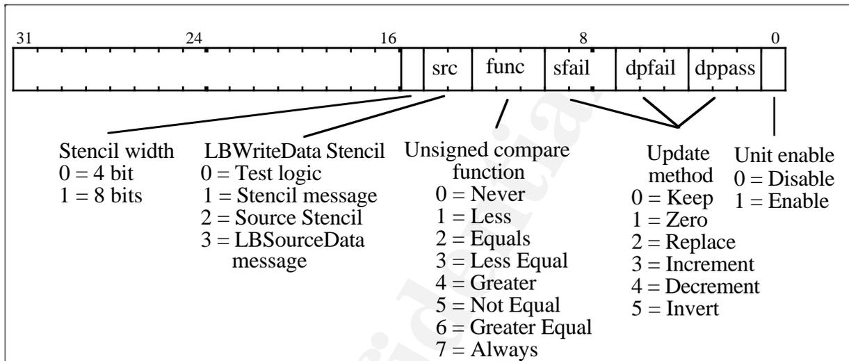
If the stencil unit is disabled then it is as if the stencil test always passes and no modification to the stencil value in the local buffer occurs. The stencil buffer *will* be updated in this situation if fast clear is enabled and the frame count is not equal.
