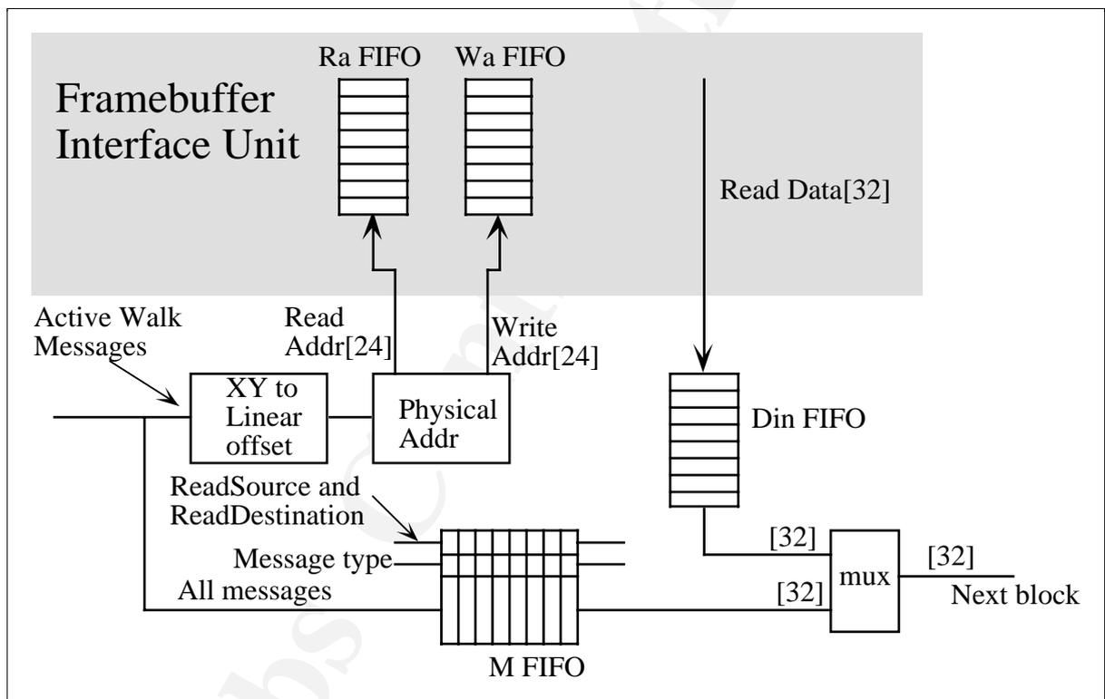
The actual reading of the memory and request arbitration is done in the Framebuffer Interface Unit.
