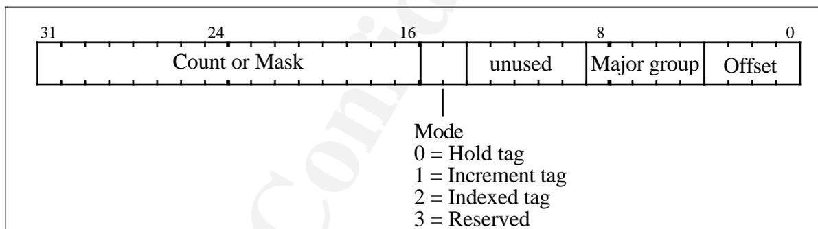
The Major group and Offset correspond to the tag table later on. The Count or Mask is a dual purpose field which is a count for Hold tag and Increment tag modes, but a mask for Indexed tag mode.
