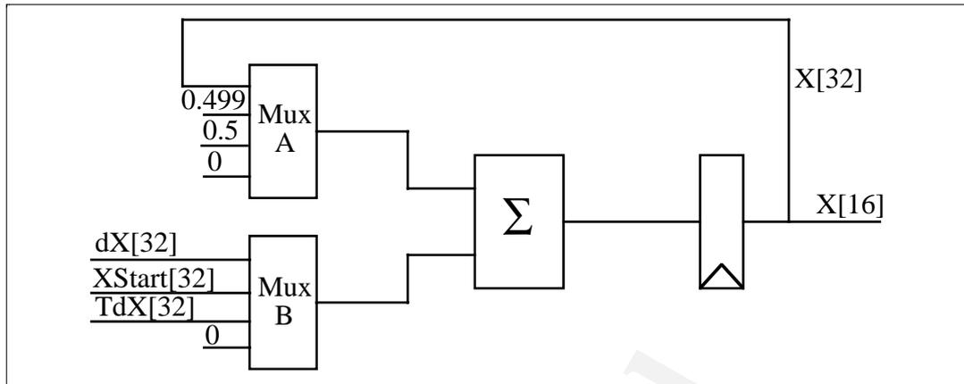
It is identical to the Y DDA unit, except for the additional input to one of the multiplexers. This takes in a delta value derived from a table, rather than a constant from a register and is used when antialiasing points. This is covered later.
