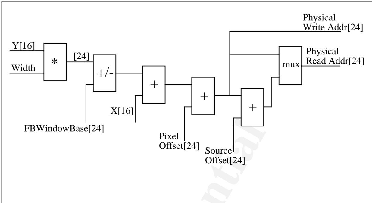
All address calculations are done to 24 bit and any overflow just wraps around. This wrap around allows  $\pm$ maximum offset to be applied with a 24 bit number. The X and Y coordinates are sign extended up to the required width.
