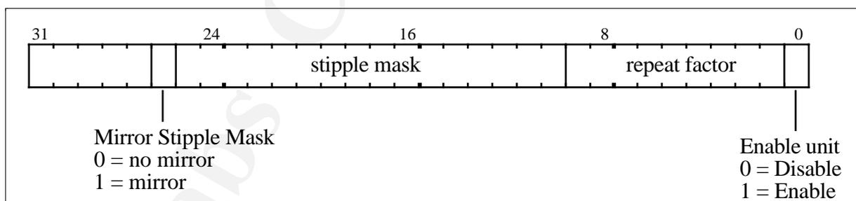
Note that the value stored as the repeat factor is one less than the desired repeat factor.
