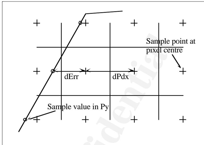
If  $dErr$  is the distance the edge is away from the pixel's centre (must be  $< 1$ ) and  $dPdx$  is the change in  $P$  for unit change in  $x$  then the correct value at the first sample point is:
