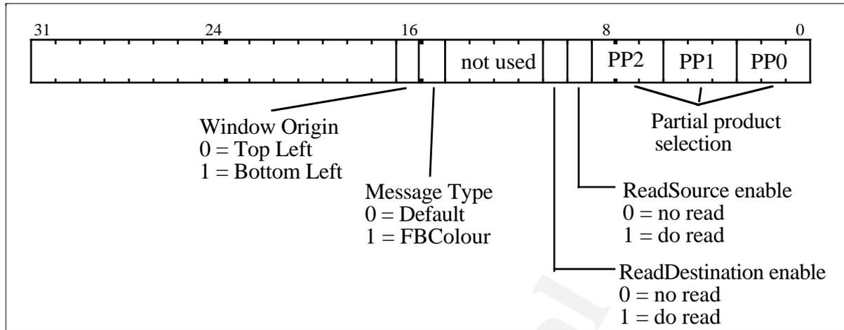
The Message Type field determines the message type the read data is encapsulated in. Normally this is Default so depending on the state of the ReadSource and ReadDestination bits the data will be sent in the FBSourceData or FBData messages respectively. For image uploads it would be FBColour.
