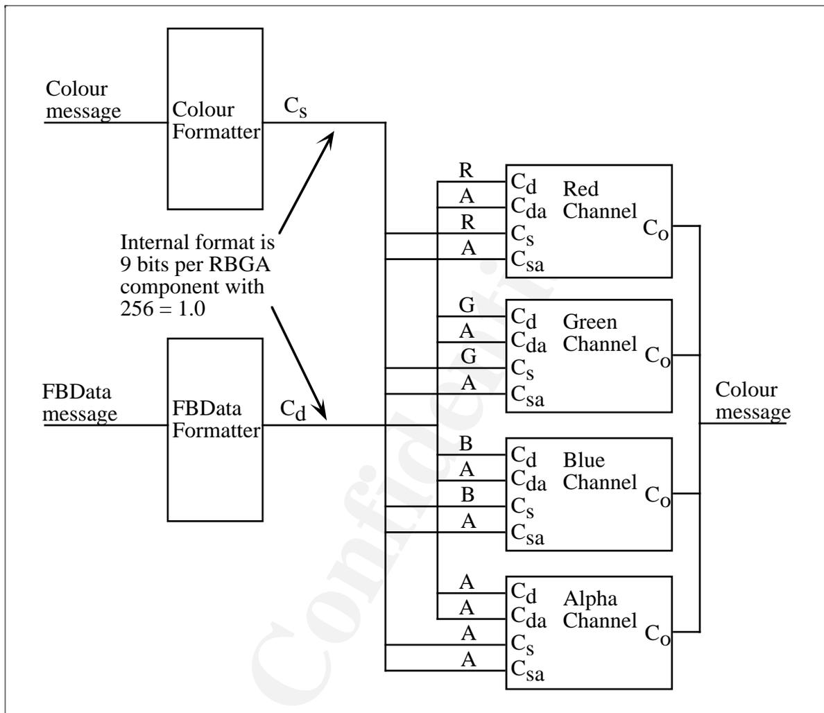
This shows the four component in a colour being processed in parallel.
