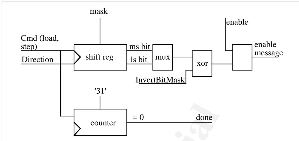
The action on each fragment is controlled by a bitmask which is rotated by one bit per fragment. If all 32 bits in the mask register have been used before the primitive has been fully rasterised the rasterisation is suspended until a new mask is loaded in. If, while waiting for a new mask, we receive any other message then the bitmaps rasterisation is aborted<sup>8</sup>. This prevents a deadlock occurring when the host doesn't send enough mask data.
