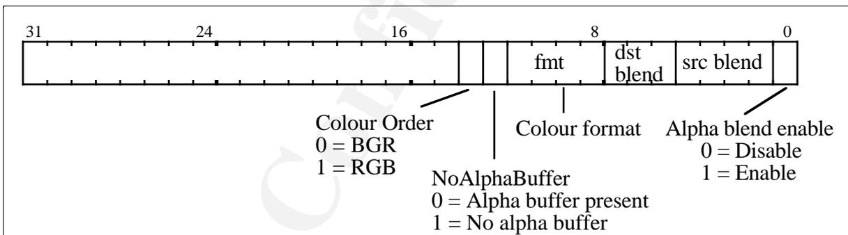
If the alpha blend is disabled then the colour message is passed through unchanged.
