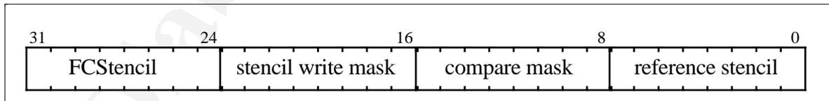
The `FCStencil` field is the stencil value which the stencil buffer would have been cleared with if the fast clear facility had not been used. This value is now substituted for the local buffer stencil value when the selected frame count is equal and Stencil FCP is enabled.
