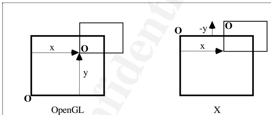
The diagram also shows that the offsets can be negative.
