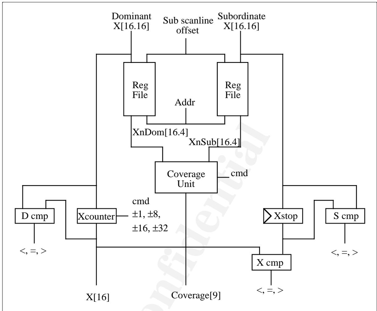
The operation of the Span Fill Unit depends on whether the trapezoid is being antialiased or not.
