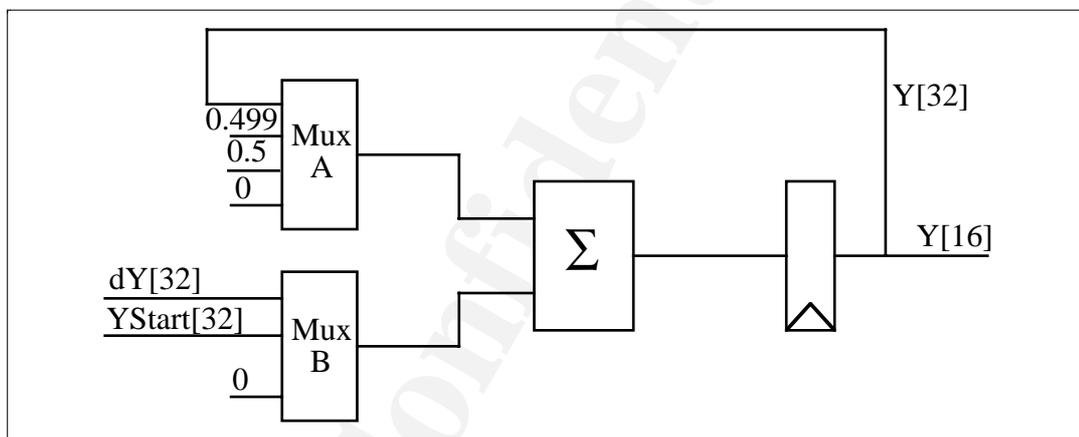
The unit responds to three commands (start, step and hold) and one of these is executed on every clock cycle. The only output value of the unit is the integer Y coordinate of the fragment or scan line we are on. Note that the direction of the step is determined by the sign of the delta Y value so it is possible to step from top to bottom, or vice versa (this flexibility is needed for line drawing and copy rectangles).
