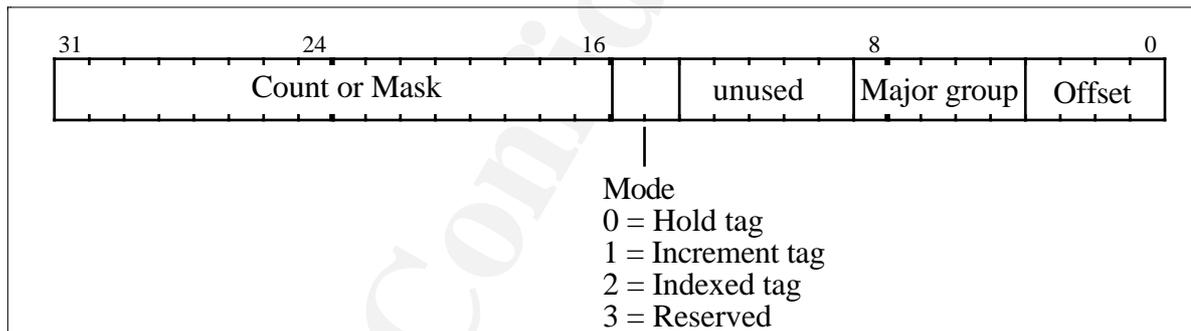
The Major group and Offset correspond to the tag table later on. The Count or Mask is a dual purpose field which is a count for Hold tag and Increment tag modes, but a mask for Indexed tag mode.
