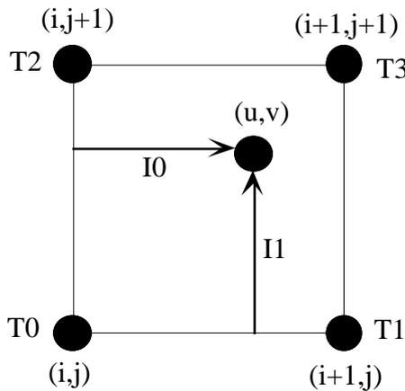
These equations are applied once for each component in the texture map. There can be 1, 2, 3 or 4 components in the texture map but as the Lerp hardware is replicated for each component this unit always works on 4 components. The same interpolation coefficient is applied to all components. It is the responsibility of the Texture Read Unit to expand fewer components into the 4 component case. This conversion is done as follows (L is luminance):
