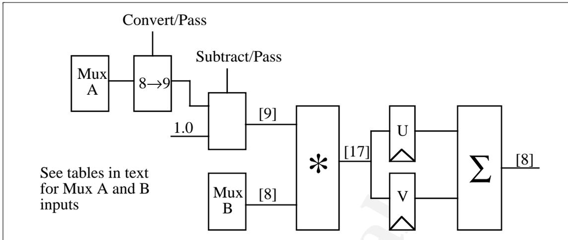
The 8→9 block will convert an 8 bit number to a 9 bit one or just pass a 9 bit one through unchanged. This is only needed when the result of the filter operation is used as the interpolation coefficient.
