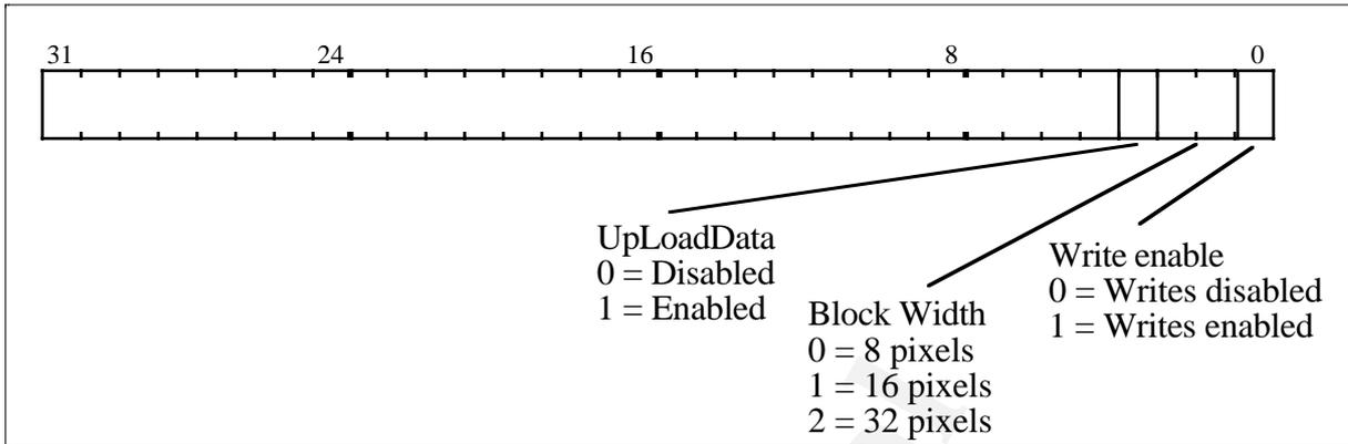
The UploadData bit, when set, causes the FBWriteData associated with each step message to be forwarded onto the next unit in a FBColour message. This feature allows data read from the framebuffer to be formatted (using the formatting logic in the Alpha Blend and Dither units) into the desired output format before being uploaded.
