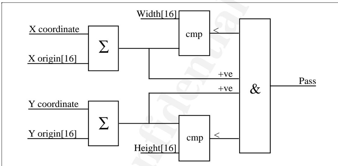
The screen and user scissor tests are controlled by the ScissorMode message, the data field of which follows.
