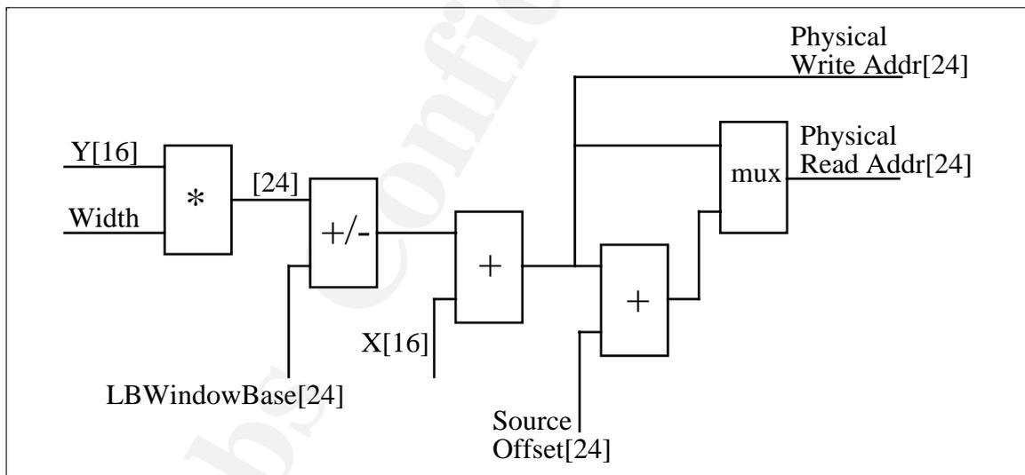
All address calculations are done to 24 bit and any overflow just wraps around. This wrap around allows  $\pm$ maximum offset to be applied with a 24 bit number. The X and Y coordinates are sign extended up to the required width.
