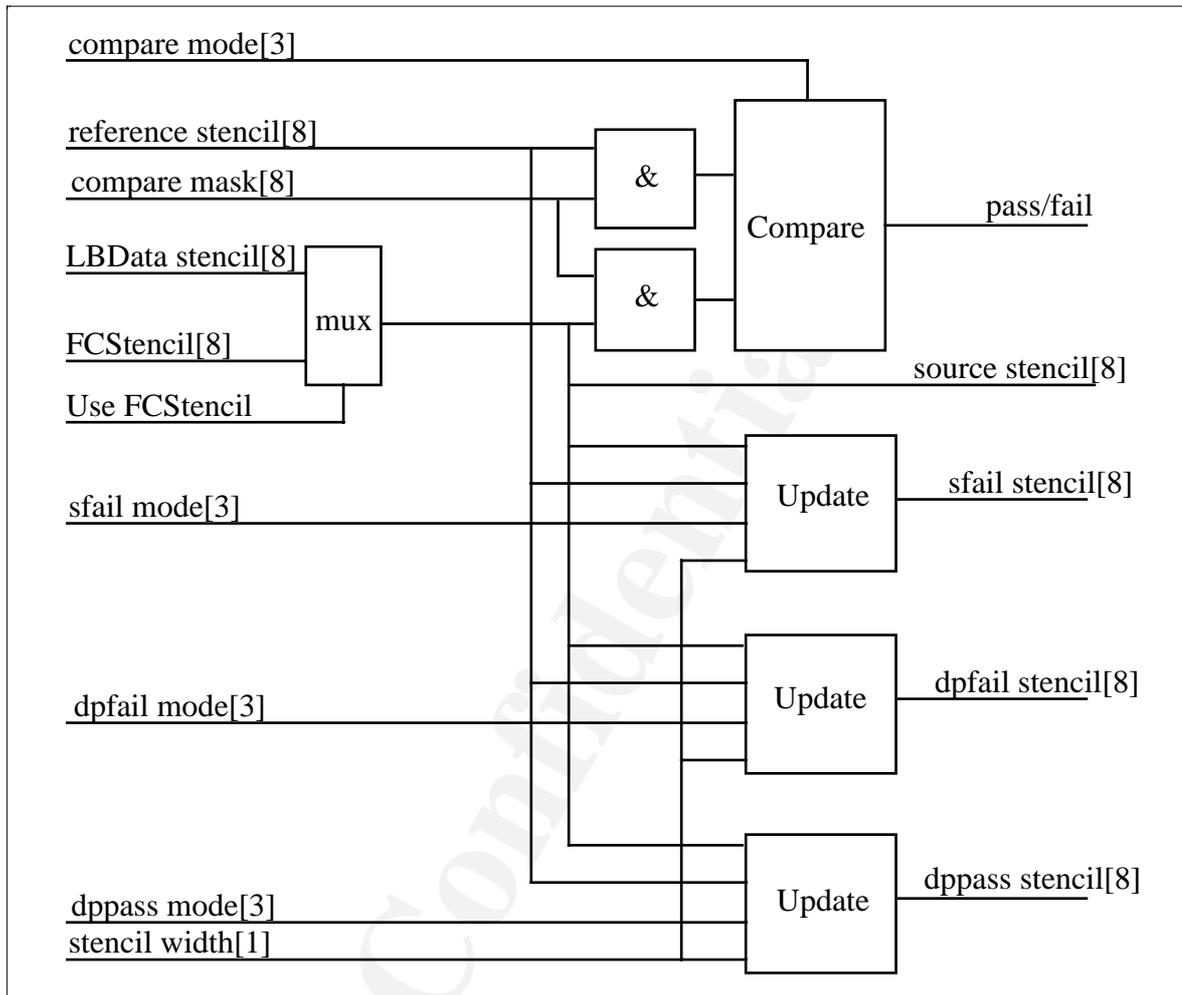
The LB stencil value is provided by the LBDData message or the Fast Clear stencil value under control of the Fast Clear logic and is subsequently called the Source Stencil. All other stencil values originate in the StencilData message and are held in the data field in the following format:
