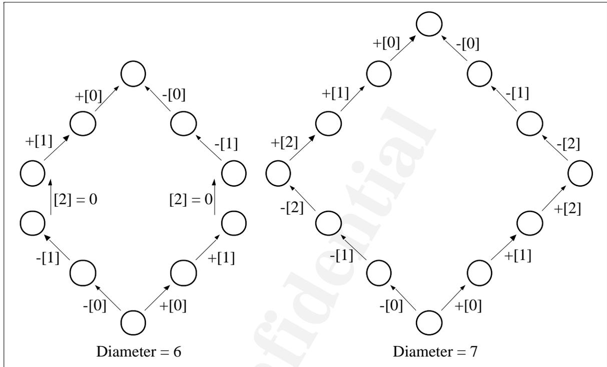
In this example the point table will have three entries. Note in the case of a even diameter the last of the required entries in the table is set to zero.
