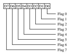
This register contains eight read-write bits which have no internal hardware function. All bits are reserved for use by BIOS and driver software.
