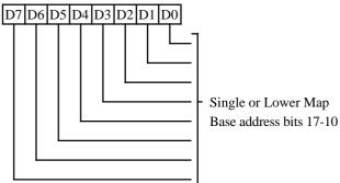
This register effects CPU memory address mapping.
