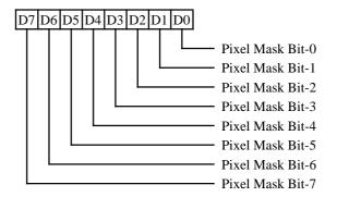
The contents of this register are logically ANDed with the 8 bits of video data coming into the color palette. Zero bits in this register therefore cause the corresponding address input to the color palette to be zero. For example, if this register is programmed with 7, only color palette registers 0-7 would be accessible; video output bits 3-7 would be ignored and all color values would map into the lower 8 locations in the color palette.
