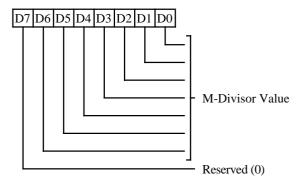
Three clock data ports (XR30-XR32) may be used to program loop parameters for loading into either the "memory" or "video" clock synthesizers. There are two sets of programmable registers, one for the Memory clock VCO and one for the Video clock VCO. The VCO currently selected for programming is determined by the Clock Register Program Pointer (XR33[5]).
