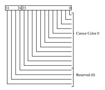
Cursor Color 0 is a 24-bit true color value consisting of 8 bits of Red, Green, and Blue. It is accessed either as two 16-bit registers or as a single 32-bit register. A write to this register immediately affects the cursor color displayed.
