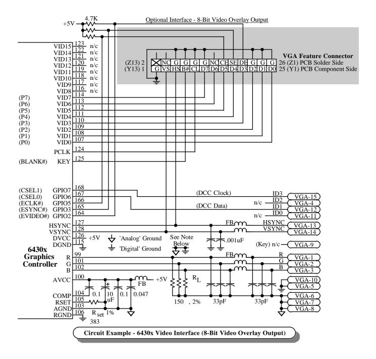
Note: The RGB DAC uses 'analog' ground as a reference; all internal digital logic uses 'digital ground' as a reference. Connections are shown separately for information purposes only. Chips and Technologies, Inc. recommends a solid ground plane for connection of all grounds.
