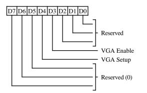
This register is accessable in all bus configurations. It is also ignored if XR70 bit-7 is set to 1 (the default is 0).
