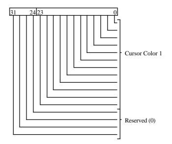
Cursor Color 1 is a 24-bit true color value consisting of 8 bits of Red, Green, and Blue. It is accessed either as two 16-bit registers or as a single 32-bit register. A write to this register immediately affects the cursor color displayed.
