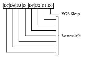
This register is only accessible in Setup Mode (enabled by register 46E8h).
