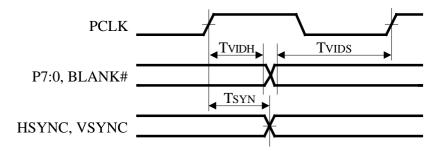
CRT Video Data and Control Signal Timing
