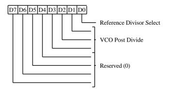
Three clock data ports (XR30-XR32) may be used to program loop parameters for loading into either the "memory" or "video" clock synthesizers. There are two sets of programmable registers, one for the Memory clock VCO and one for the Video clock VCO. The VCO currently selected for programming is determined by the Clock Register Program Pointer (XR33[5]).
