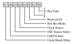
These bits latch the state of MAD7:0 on the falling edge of RESET. The state of bits 7:0 after RESET effect chip internal logic as indicated below. MAD7:0 have no on-chip pullups or pull-downs; therefore, the state of these bits after RESET will be indeterminate if no external pullup or pulldown resistors are present.
