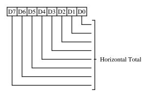
7-0 Horizontal Total. Total number of character clocks per line = contents of this register + 5. This register determines the horizontal sweep rate.
