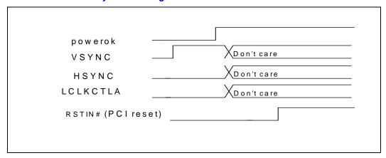
NOTE: VSYNC and LCLKCTLA = ALL Z Test Mode Activation; No clock is required for ALLZ Test Mode Activation. A minimum of 50 ns PWROK assertion prior to RSTIN# assertion is recommended. A minimum of 10 ns VSYNC/HSYNC/LCLKCTLA assertion prior to PWROK assertion is recommended.
