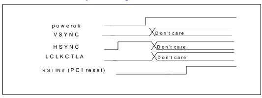
NOTE: HSYNC and LCLKCTLA = XOR Chain Test Mode Activation; No clock is required for XOR Chain Test Mode. A minimum of 50 ns PWROK assertion prior to RSTIN# assertion is recommended. A minimum of 10 ns VSYNC/HSYNC/LCLKCTLA assertion prior to PWROK assertion is recommended.
