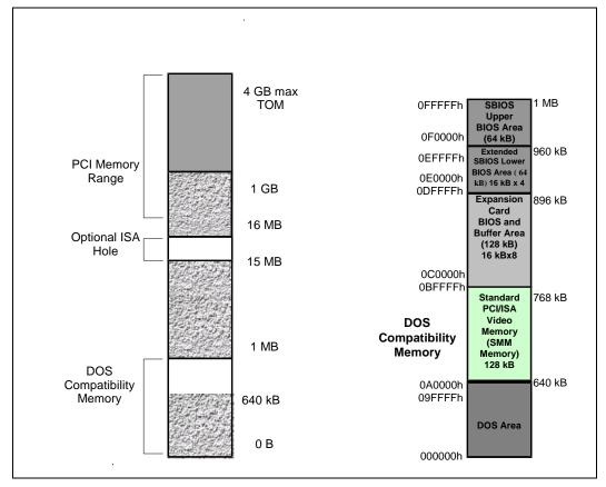
Figure 7. Detailed View of System Address Map
