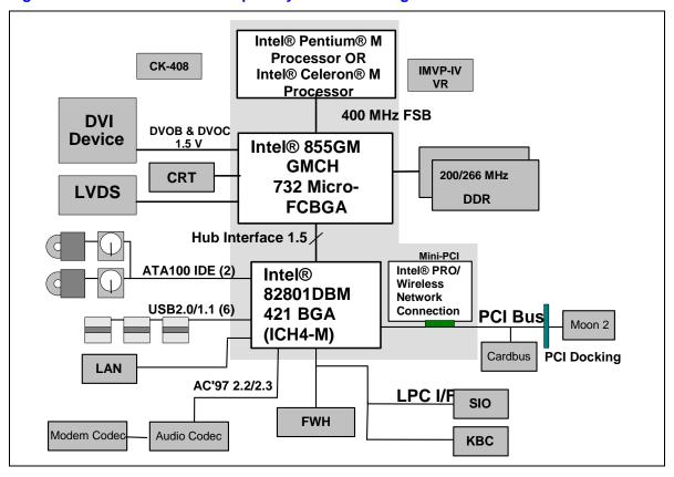
Figure 1. Intel® 855GM GMCH Chipset System Block Diagram
