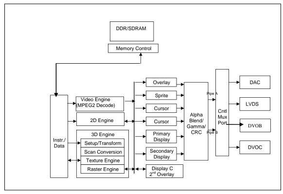
Figure 8. Intel® 855GM GMCH Graphics Block Diagram
