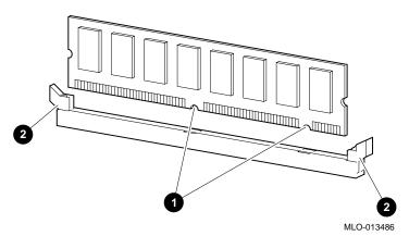
Figure 2–2 Installing PowerStorm 4D40T/4D50T/4D60T Texture Memory
