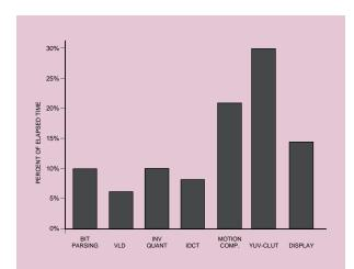
Figure 7. Where the Time is Spent. MPEG-1 (SIF Resolution 352 x 240) at 30 fps on 275 MHz Alpha AXP<sup>1</sup>
