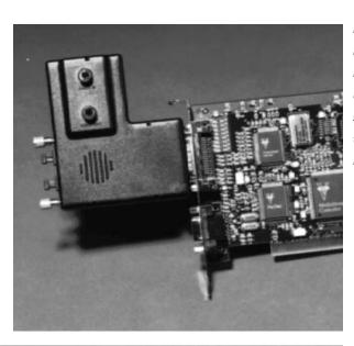
Figure 17. BtV MediaStream Family's unique breakout adapter shown connected to the BtV2100EVK PCI card.
