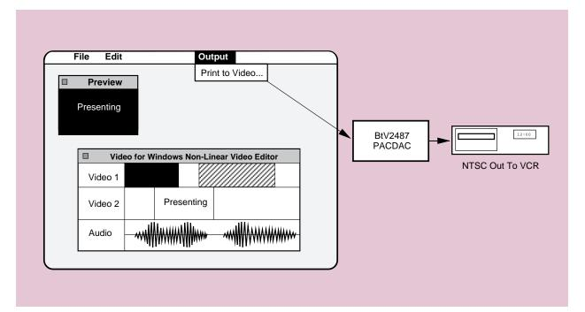
Figure 12. Typical Print-to-Video NTSC/PAL Encoding Example
