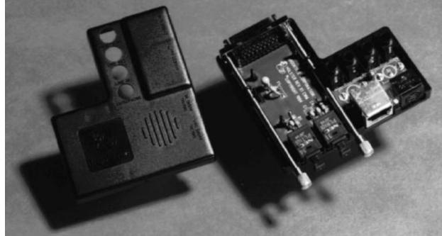
Figure 18. The A/V breakout adapter provides an external carrier of the connectors needed for the audio and video features.
