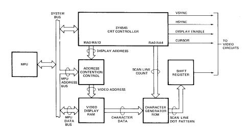
Figure 5. Shared Memory System Configuration
