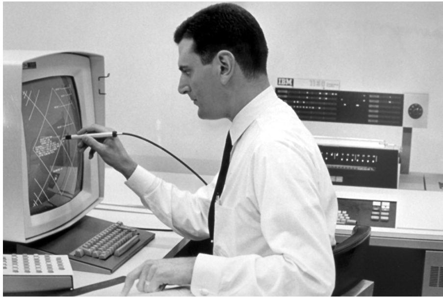
Figure 13.5 IBM 2250 Display Connected to an IBM 1130 Computer 8
