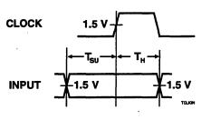
Figure 4-2. Input Timing
