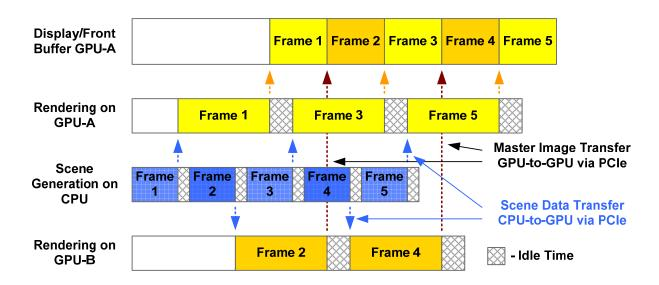
Figure 3. Alternate Frame Rendering (AFR) Activity Example Timeline
