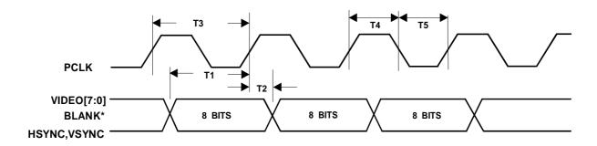
Figure 8.11 Video Timing 4, 8, and 16 Bits/Pixel Modes
