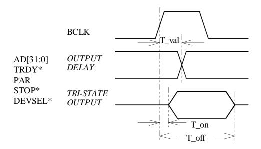
Figure 8.2 PCI/AGP Output and Tri-state Timing
