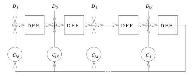
Figure 4.5 Multi-Input Signature Register (MISR)
