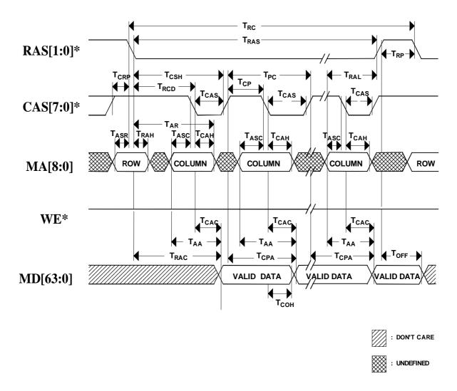
Figure 8.9 Video Memory Fast Page Mode Read Cycle with Extended Data
