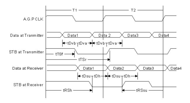
Figure 8.4 AGP 133 Timing Diagram
