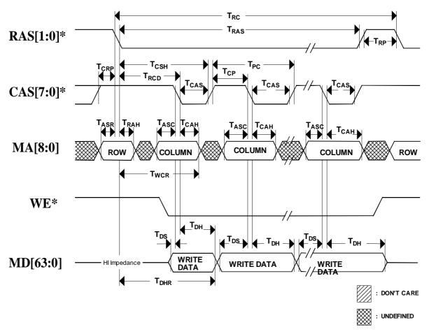
Figure 8.8 Video Memory Fast Page Mode Write Cycle
