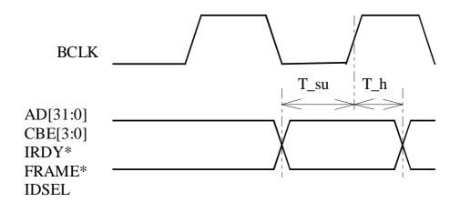
Figure 8.3 PCI/AGP Input Timing
