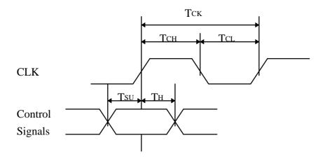
Figure 8.10 SDRAM/SGRAM input/output Timing
