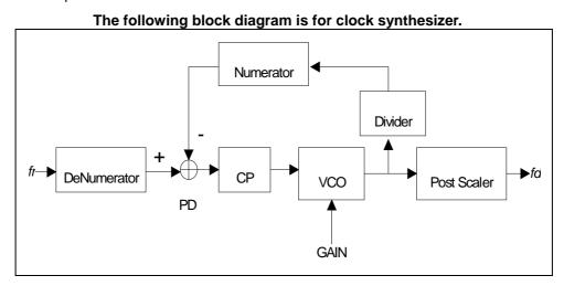
Figure 2.15 -1 Block Diagram of Clock Synthesizer
