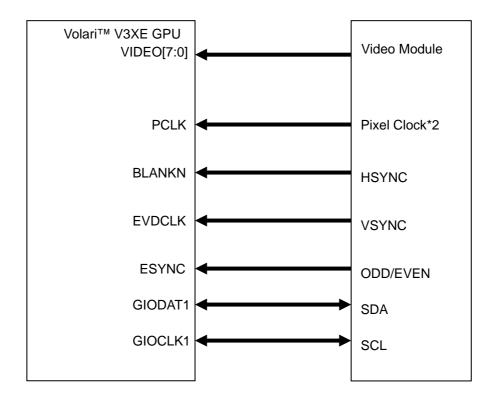
The video input interface could capture one of RGB565, YUV422 or YUV420 video data format and store the video data into the video frame buffer. The new YUV420 mode could reduce the video capture bandwidth and video capture frame buffer size. The video input unit also provides the horizontal and vertical downscaling filter to generate better video capture quality. The vertical downscaling filter is implemented by a video capture frame buffer read back operation (no line buffer is required).
