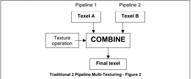
Traditional 2 Pipeline Multi-Texturing - Figure 2 shows a dual-pipeline on a traditional hardware renderer.
