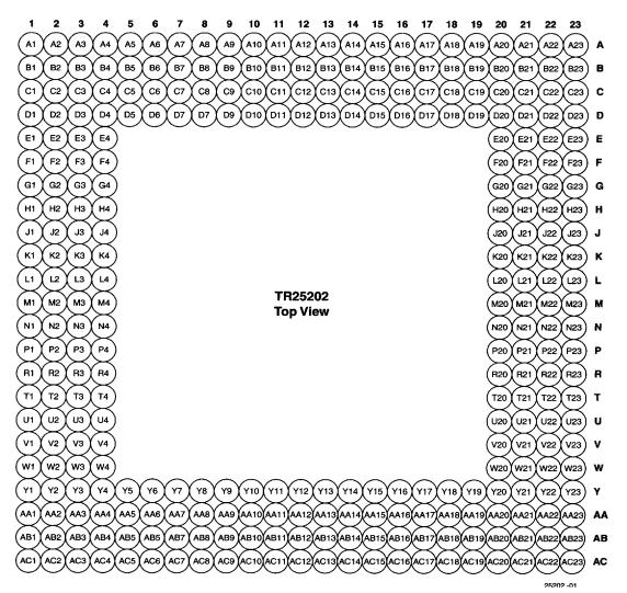
Figure 1 • TR25202 Pinout (Top View)
