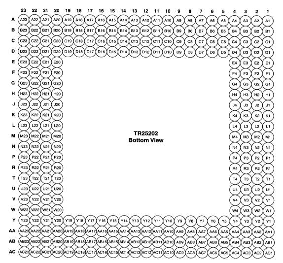
Figure 2 • TR25202 Pinout (Bottom View)
