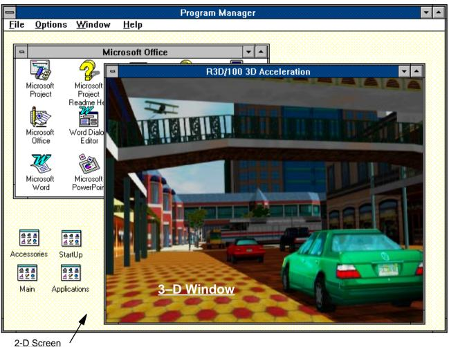
Figure 1. 3-D Rendering Window within 2-D Screen
