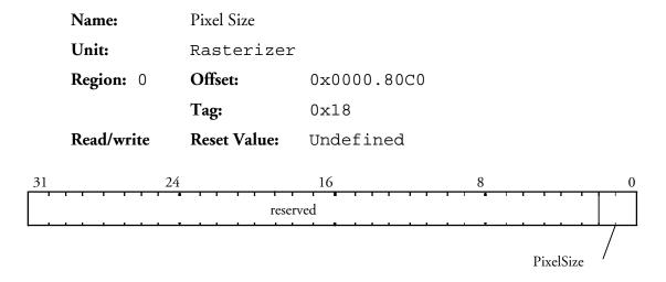
Configures the pixel depth to be used for rendering.
