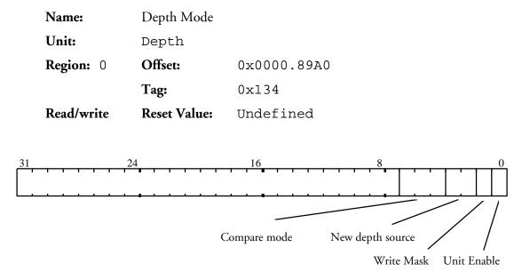
Controls the comparison of a fragment's depth value and updating of the depth buffer. If the compare function is LESS and the result is true then the fragment value is less than the source value.
