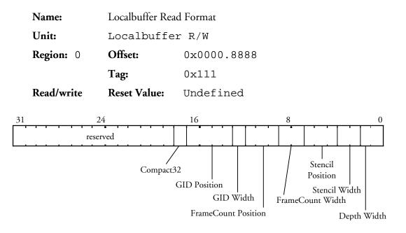
Specifies the format used when reading from localbuffer memory. The effect of creating a format with overlapping fields is undefined.
