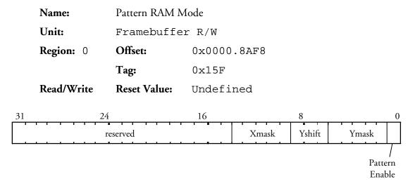
Holds the mode information when the Pattern RAM is used as the source of data during a span operation.
