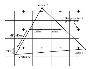
The vertices are sorted into Y order and the dominant edge is AC. Scan conversion will start at vertex A and proceed upwards. The origin is bottom left.
