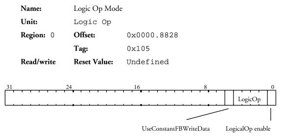
Controls Logical Operations on the framebuffer.
