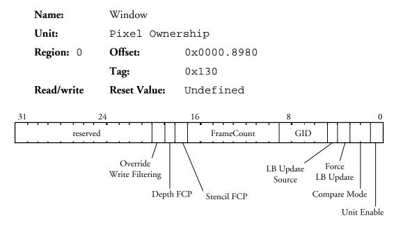
Used to set the value and comparison mode for the pixel ownership (GID) test. If the test fails then the fragment will be culled from being drawn.
