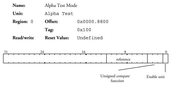
When the unit is enabled, the compare operation compares the fragment's alpha value, against the reference alpha value in this register. If the comparison result is false, then the fragment is culled, and will not be drawn.
