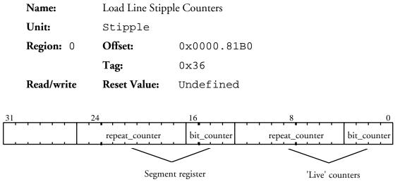
Command register used to restore the line stipple counters and segment register after a task switch. The counters are incremented during a line stipple so the value read from them, via the read back path may not match the value loaded into them using this register.
