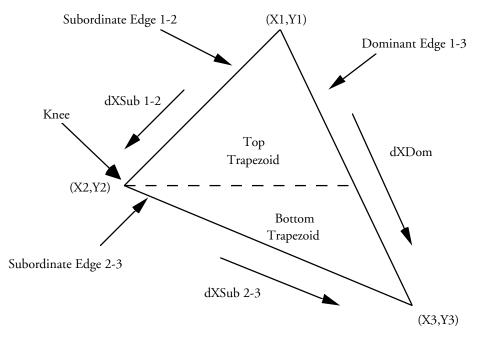
Figure 0.5 Rasterizing a triangle.
