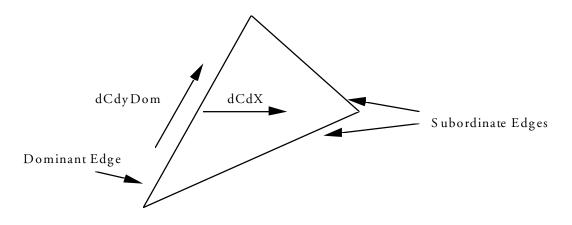
dCdyDom = color gradient in the Y direction along the dominant edge dCdx = color gradient in the X direction
