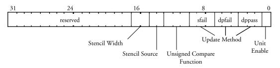
Controls the stencil test, which conditionally rejects fragments based on the outcome of a comparison between the value in the stencil buffer and a reference value in the StencilData register. If the test is LESS and the result is true then the fragment value is less than the source value.
