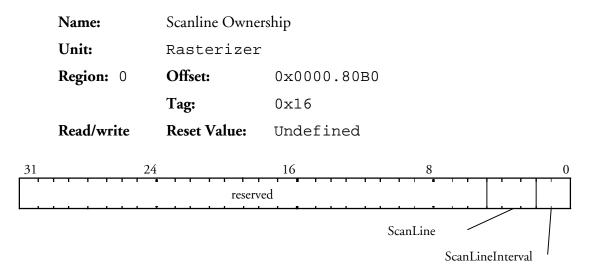
Controls which scanlines a GLINT owns in a multi-GLINT system. This register only has an effect if the MultiGLINT bit is set in the **RasterizerMode** register.
