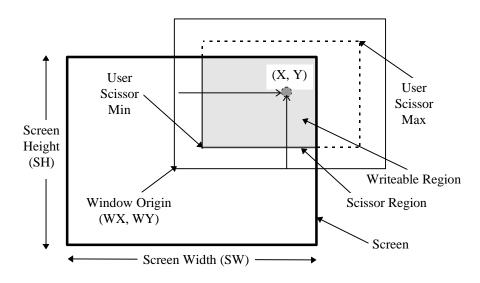
Figure 0.12 Screen Scissor and User Scissor Tests
