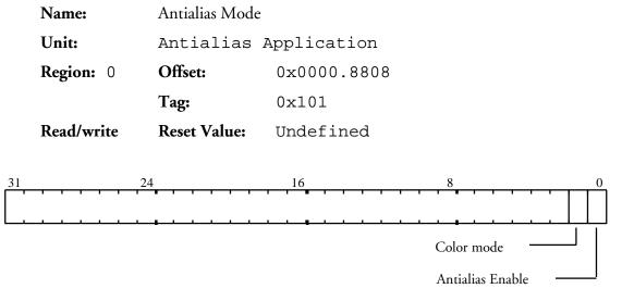
Controls the operation of antialiasing. When the unit is enabled:
