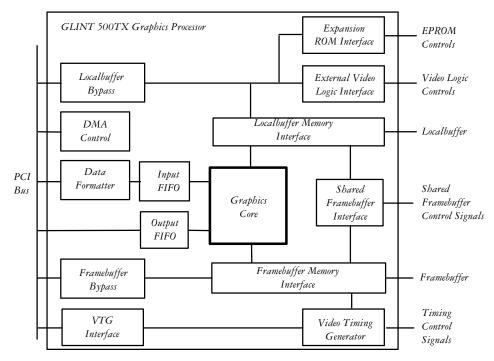
Figure 0.1 High level blocks in the GLINT architecture
