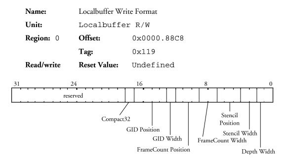
Specifies the format used when writing to localbuffer memory. The effect of setting a configuration with overlapping fields is undefined.
