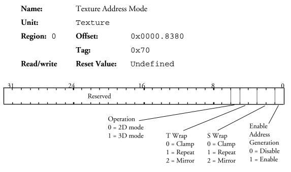
Provides overall control of the generation of texel addresses.
