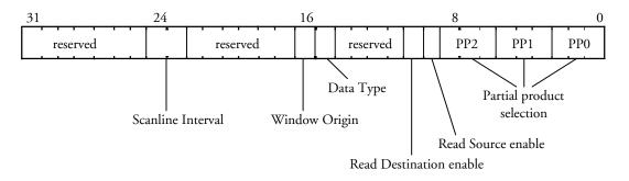
Figure 0.43 FBReadMode Register
