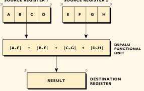
SPECIAL MULTIMEDIA OPERATIONS The ume8uu operation, commonly used for motion estimation in video compression, implements 11 simple operations in one TriMedia special op.
