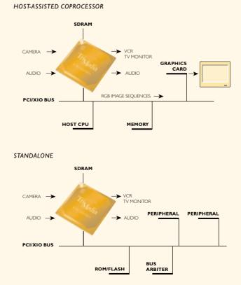
TM-1300 is designed for use as the sole CPU in standalone systems and as a coprocessor in a hosted or multiprocessor environment.
