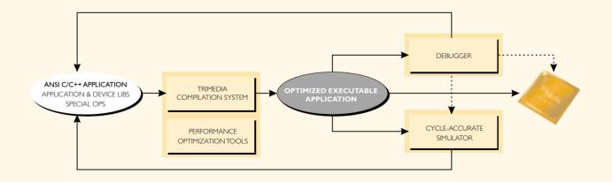
The TriMedia Software Development Environment includes a full suite of system software tools to compile and debug code, analyze and optimize performance, and simulate execution on TriMedia processors.
