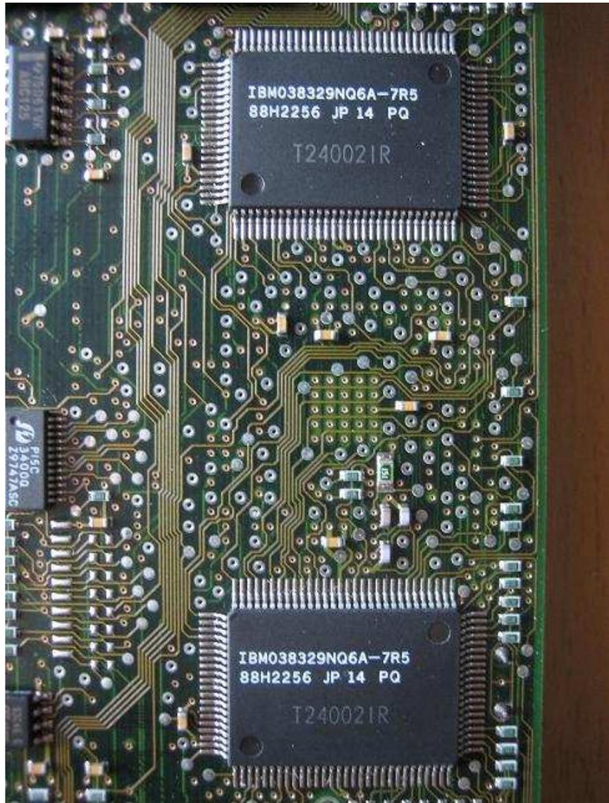
Located in the back of the card2starsPQFPpackage,IBM SGRAMmemory, chip size1 MB,7.5ns, the maximum operating frequency of133MHz, specifically forPERMEDIA 2 Vgraphics chips to use.
