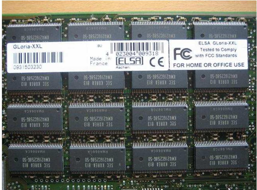
16MBframe buffer, from both sides of the 16 films threestars256K X 16 VIDEO RAM composed of single size 512KB, 50ns, used to store frame buffer data. Memory is also posted on the ELSA model label, you can see in the above graphics origin is France.
