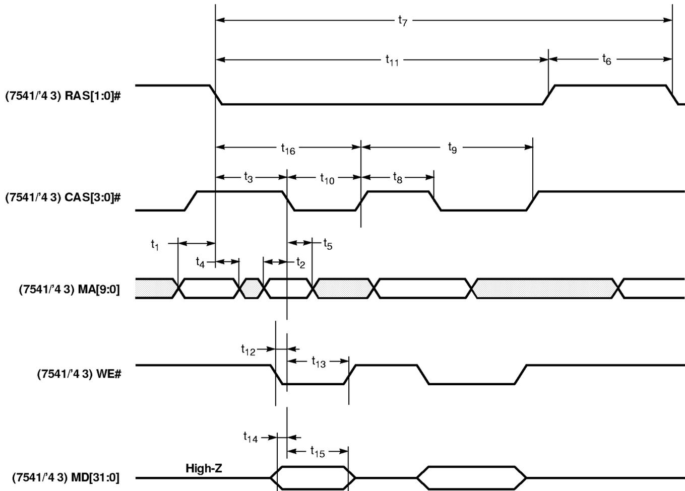
Figure 13-16. Display Memory Bus — Write Timing
