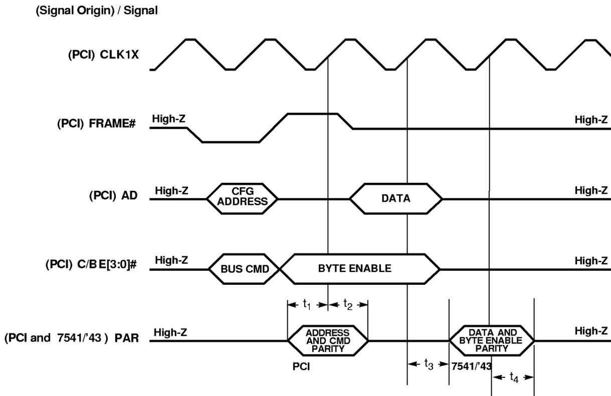
**Figure 13-14. PCI Bus — PAR Timing (Read )**
