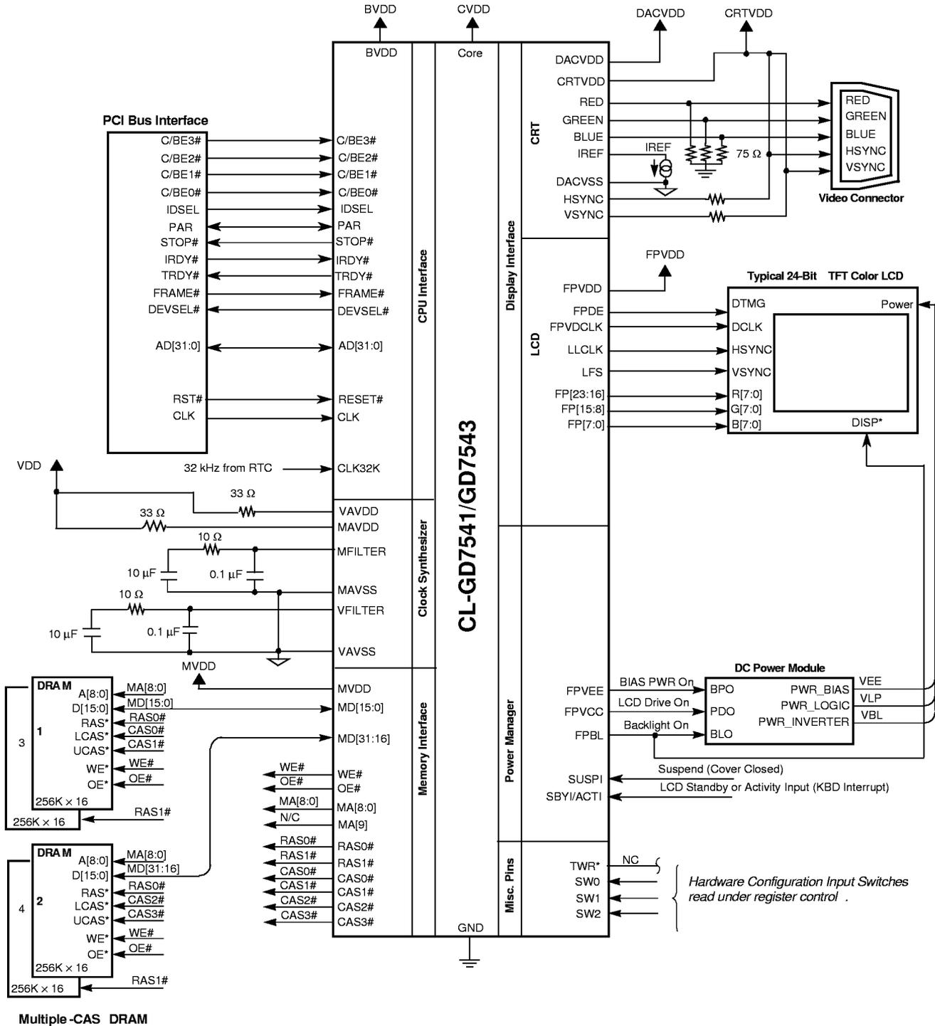
**1.3.6 PCI Bus, 1-Mbyte 256K × 16 DRAM, 18-Bit TFT Color, Feature Connector Interface**
