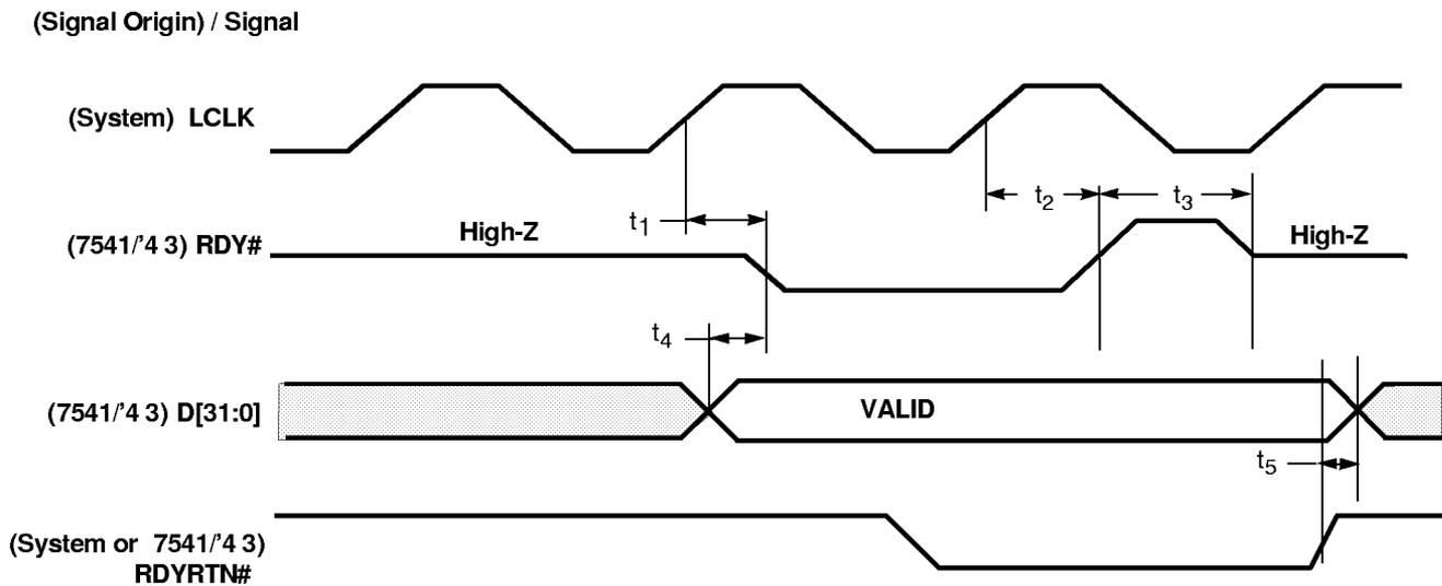
**Figure 13-4. Local Bus — RDY# and Read-Data Timing**
