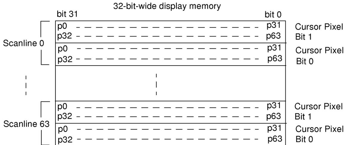
**Figure B-2. Mapping of 64 × 64 Hardware Cursor**
