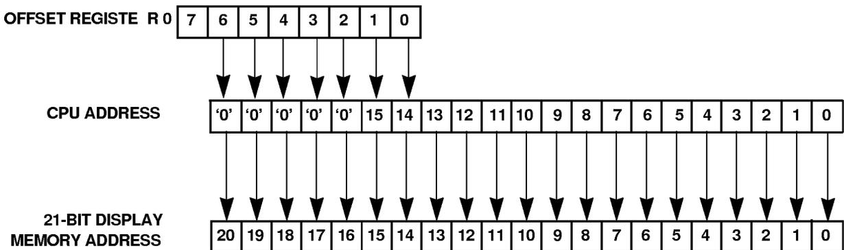
**Figure K-9. 64K Page-Mode Remapping Address Alignment for 2-Mbytes Memory**
