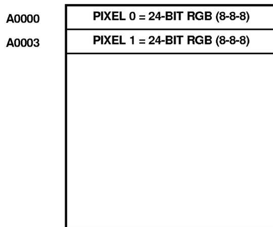
**Figure K-6. 24-Bit True Color Packed-Pixel Mode**
