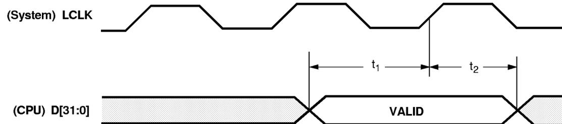
Figure 13-6. Local Bus — Write Data Timing
