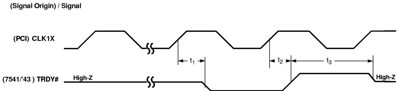
**Figure 1 3-9. PCI Bus — TRDY# Delay Timin g**
