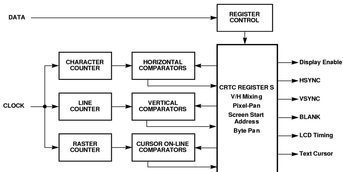
Figure 3-5. CRT Controller Functional Block Diagram
