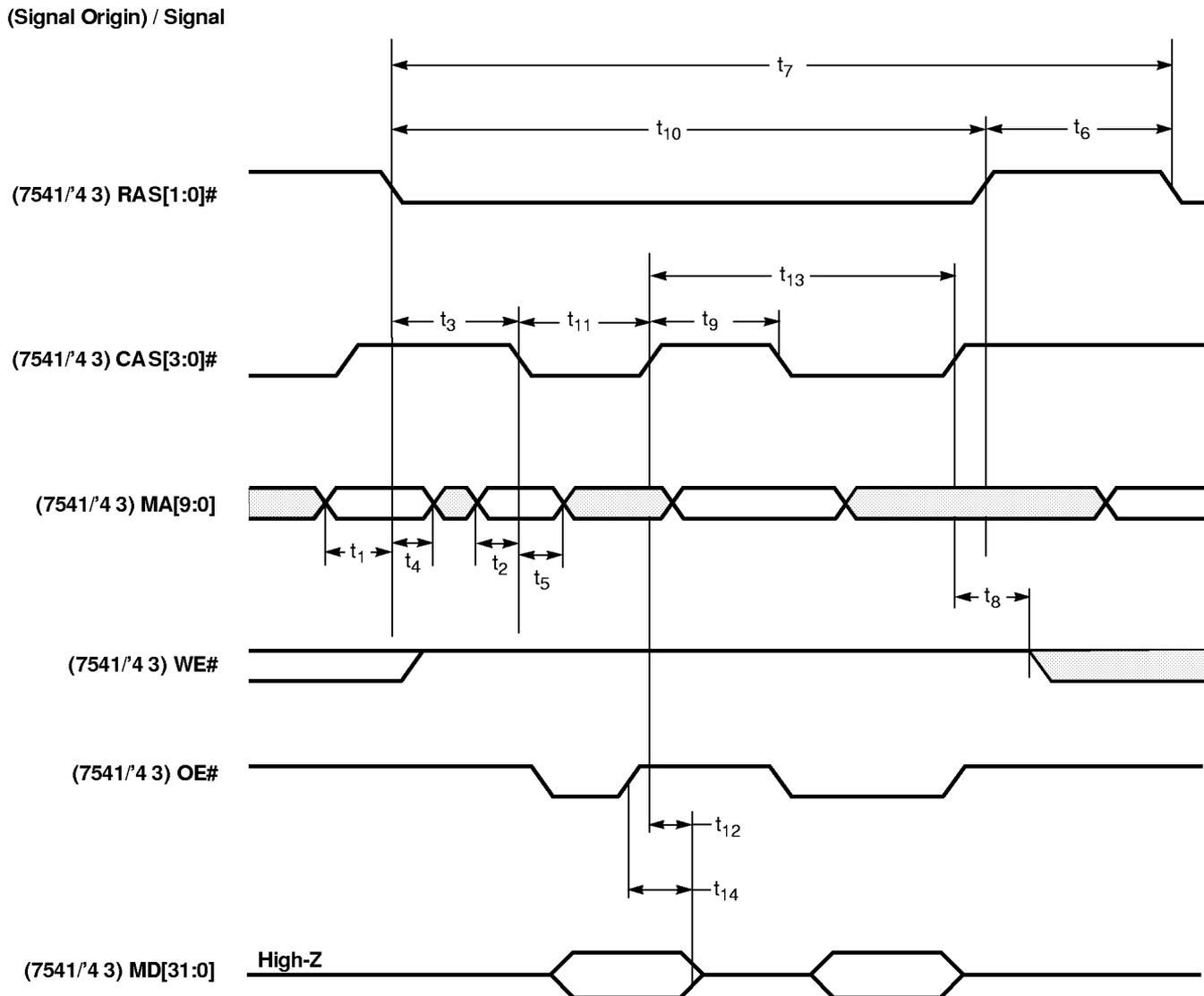
Figure 13-15. Display Memory Bus — Read Timing
