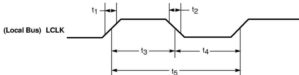
**Figure 13-2. Local Bus — LCLK Timing**
