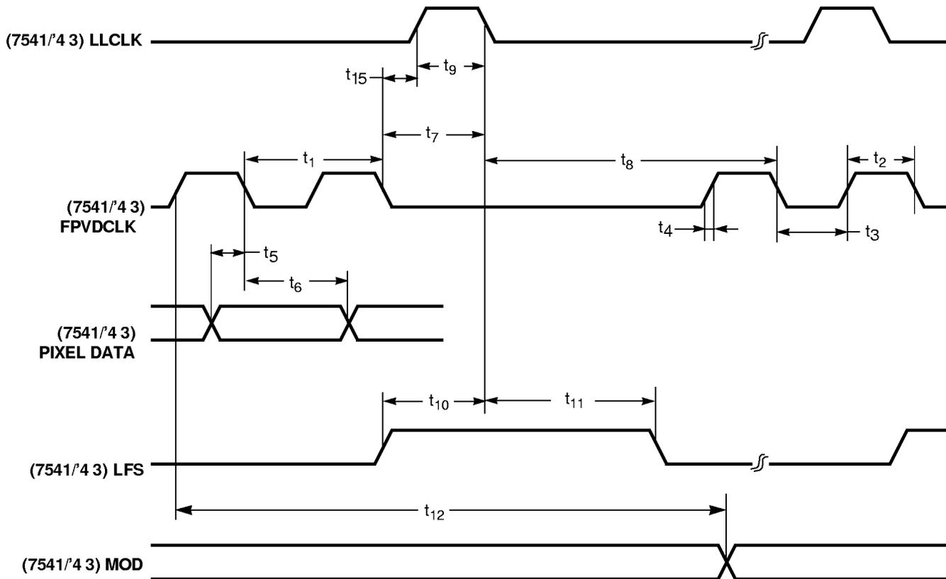
Figure 1 3-20. LCD Interface — Timing for STN Monochrome and Color-Passive LC D
