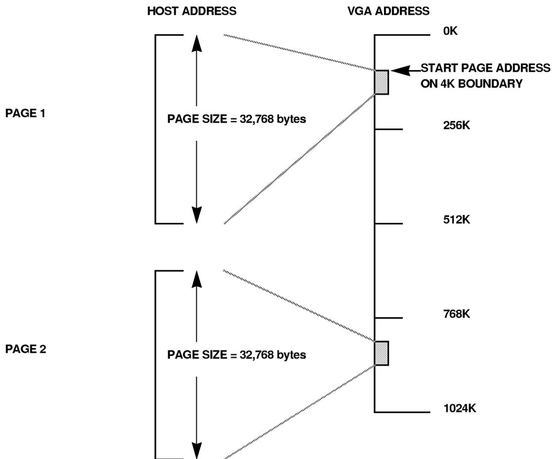
Figure K-10. Dual-Page Address Mapping Scheme
