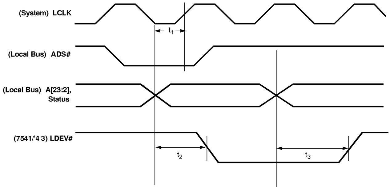
**Figure 13-3. Local Bus — ADS# and LDEV# Timing**
