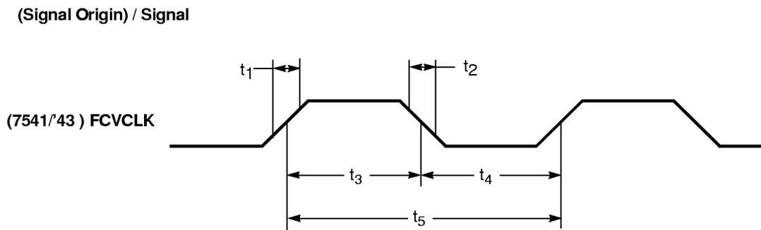
**Figure 13-19. Feature Connector — FCVCLK Input Timing Requirement s**
