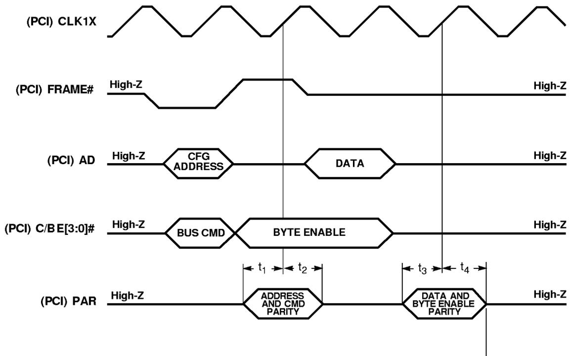
**Figure 13-13. PCI Bus — PAR Timing (Write )**
