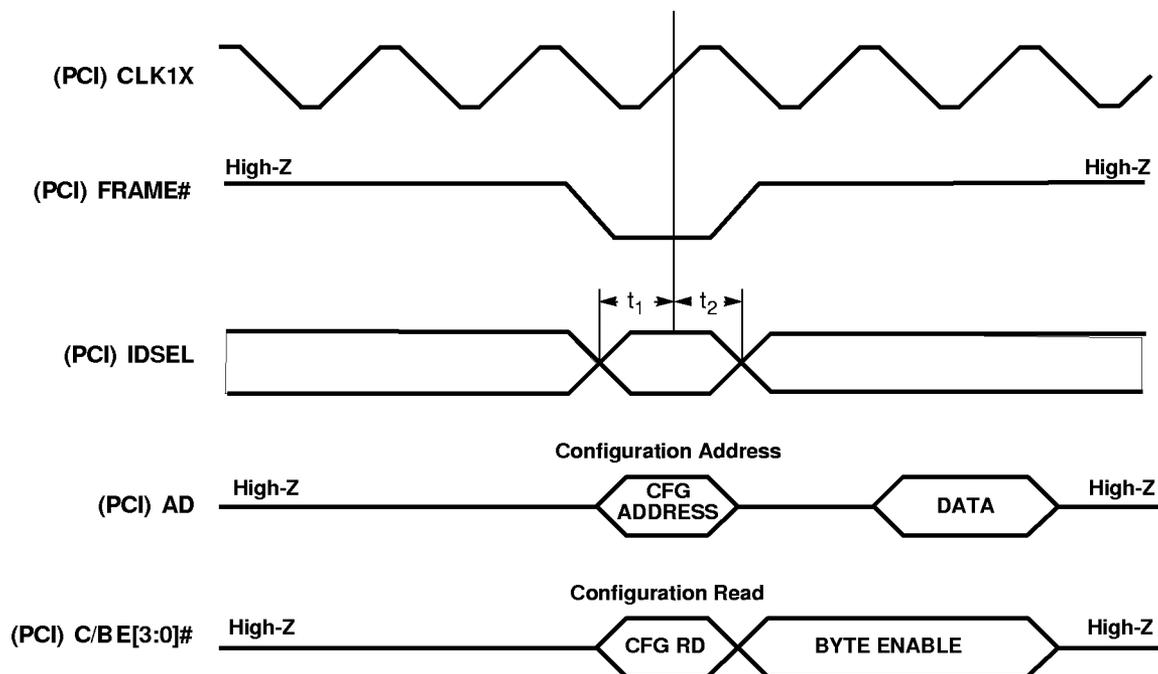
**Figure 13-12. PCI Bus — IDSEL Timing**
