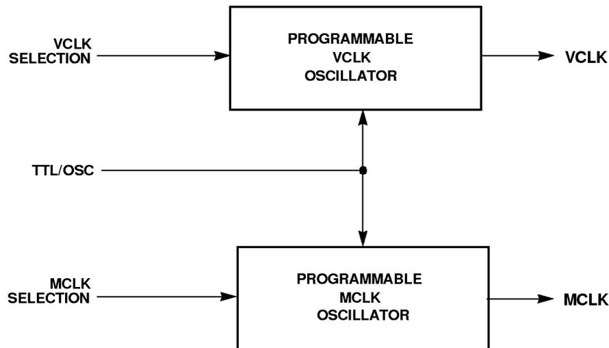
Figure 3-10. Programmable Dual-Frequency Synthesizer Functional Diagram
