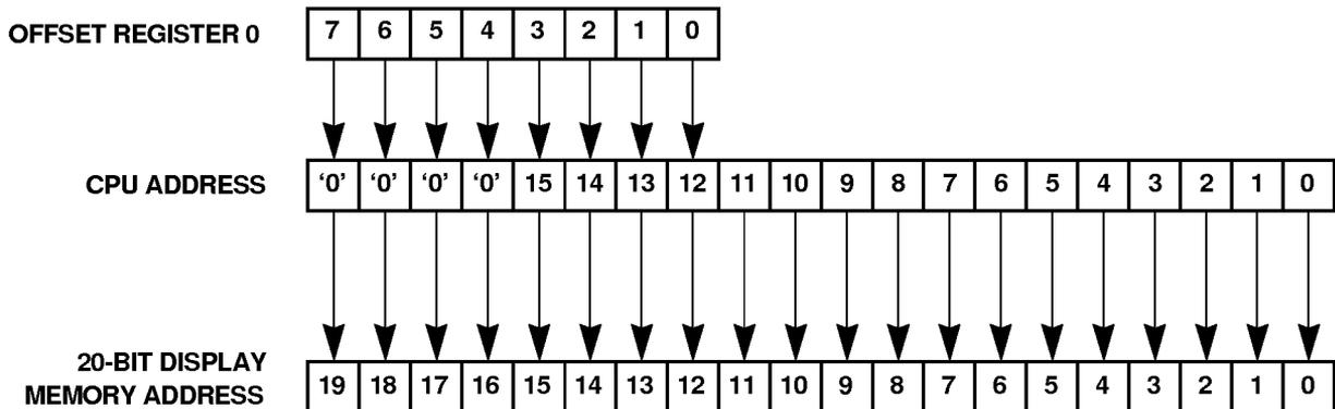
**Figure K-8. 64K Page-Mode Remapping Address Alignment for 1-Mbyte Memory**
