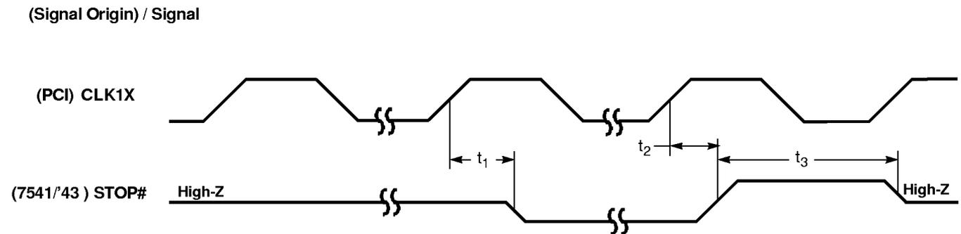
**Figure 13-11. PCI Bus — STOP# Delay Timing**
