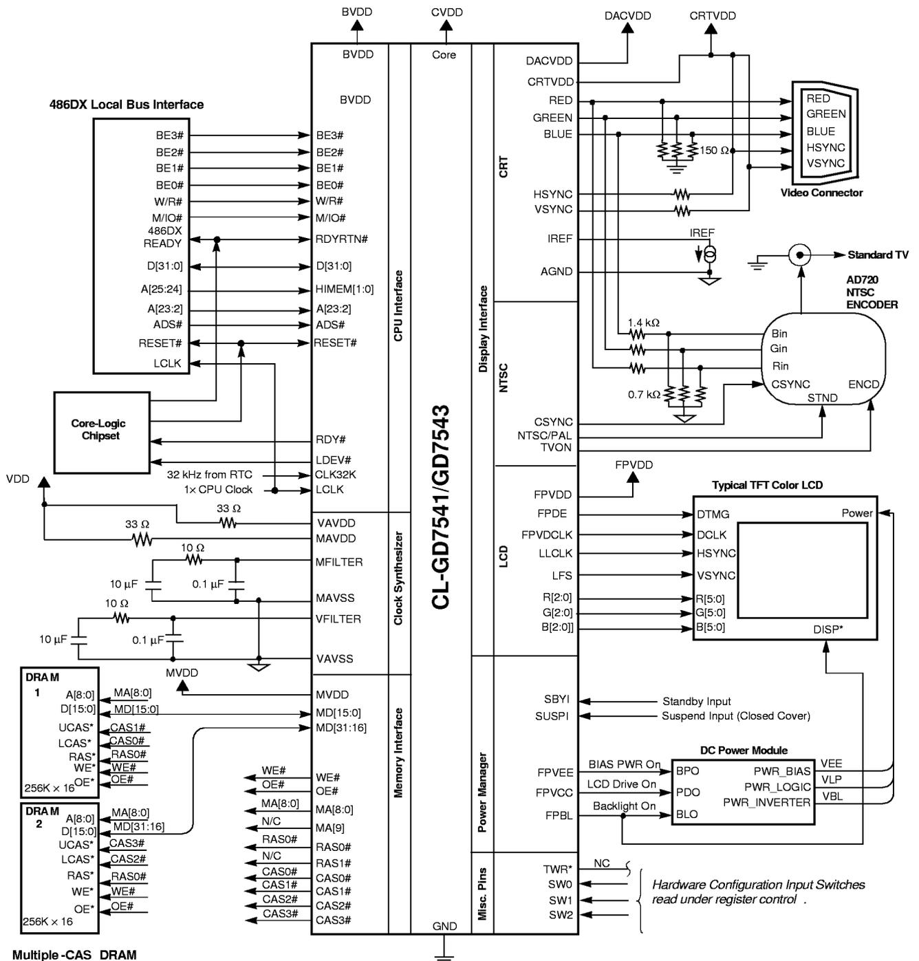
NOTE: When using the design featured in this diagram, the CRT must be disconnected when using the NTSC output.
