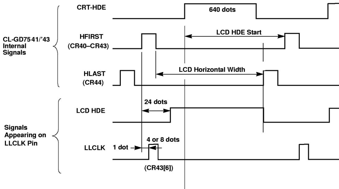
**Figure 1 2-4. Horizontal Position for STN LCD Displaying 640 × 480 Picture**
