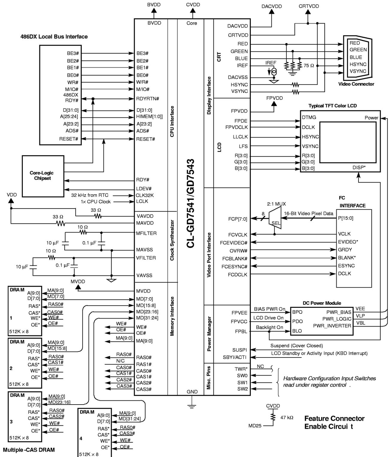
**1.3.2 Local Bus (32-Bit '486DX or VES A® VL-Bus™), 1-Mbyte 256K × 16 DRAM, 8-Bit Dual-Scan Monochrome**
