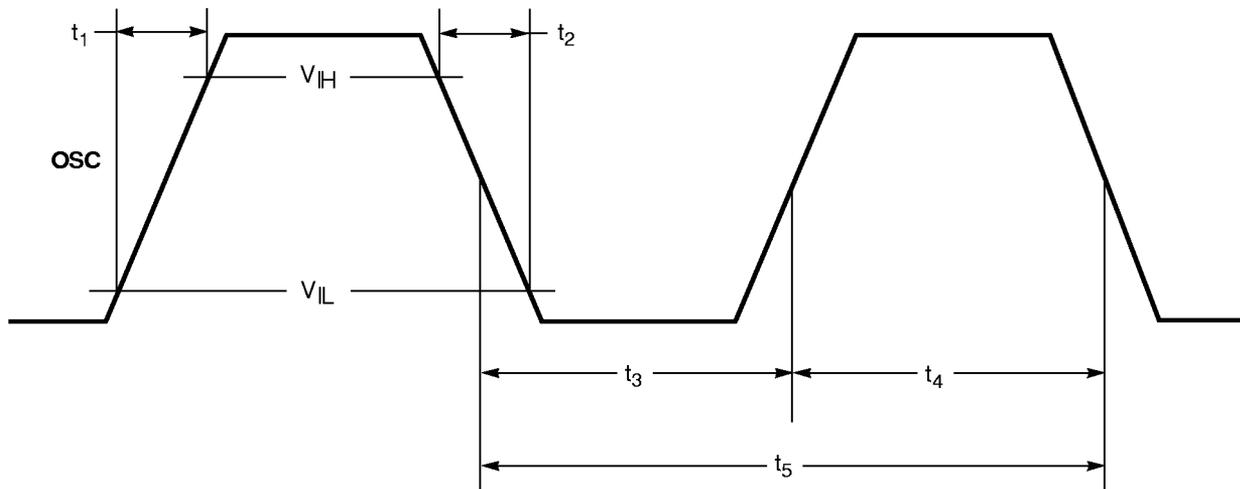
**Figure 13-22. Frequency Synthesizer — Input Timing**
