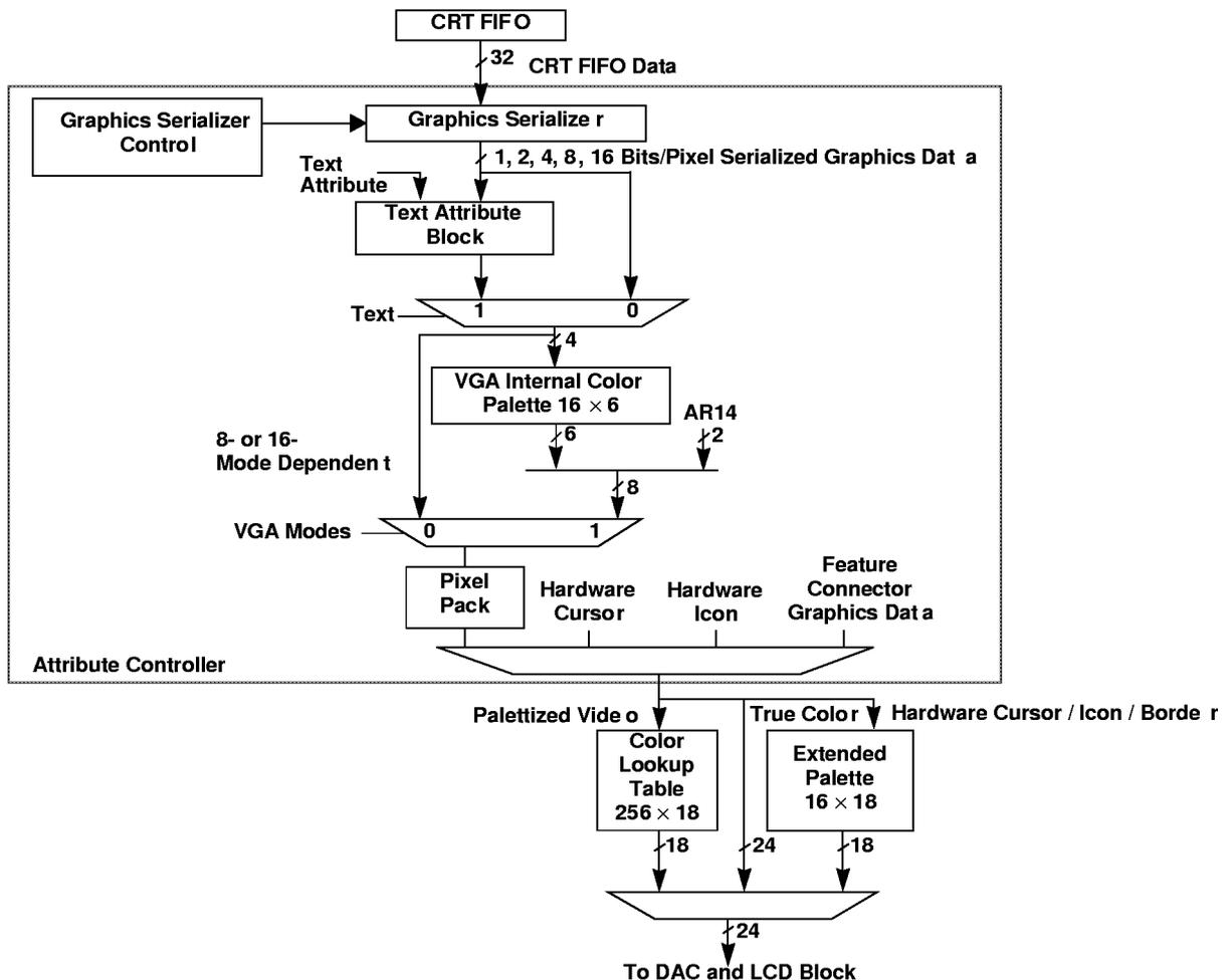
Figure 3-4. Attribute Controller Functional Block Diagram
