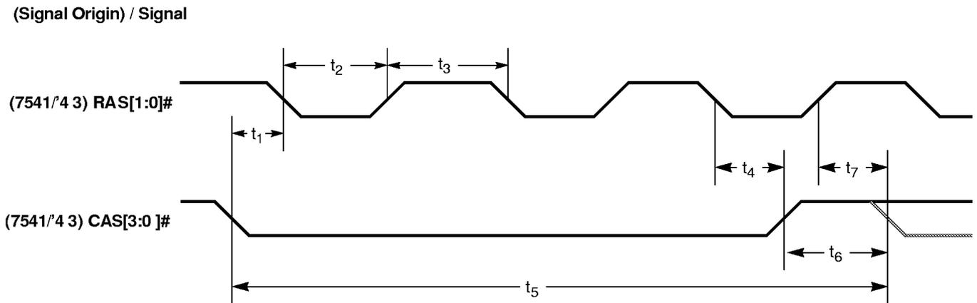
**Figure 13-17. Display Memory Bus — CAS#-before-RAS# Refresh Timing**
