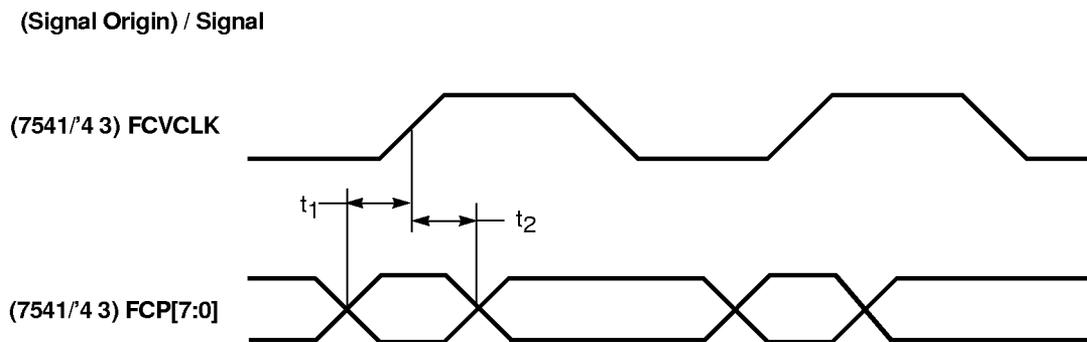
**Figure 13-18. Feature Connector — Timing with Clock and Data Driven Externally**
