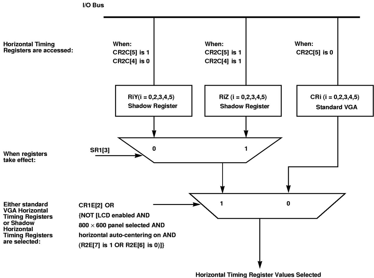
Figure 1 2-2. Horizontal Timing Register Values Selection
