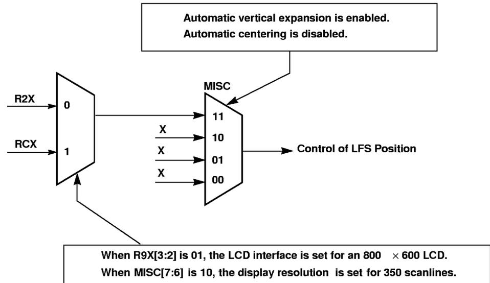
**NOTE:** For 800 × 600 and 640 × 480 LCDs, the vertical expansions are controlled by different bits, and the expansion algorithms are different.
